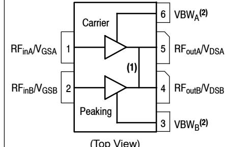
Figure 1. Pin Connections
