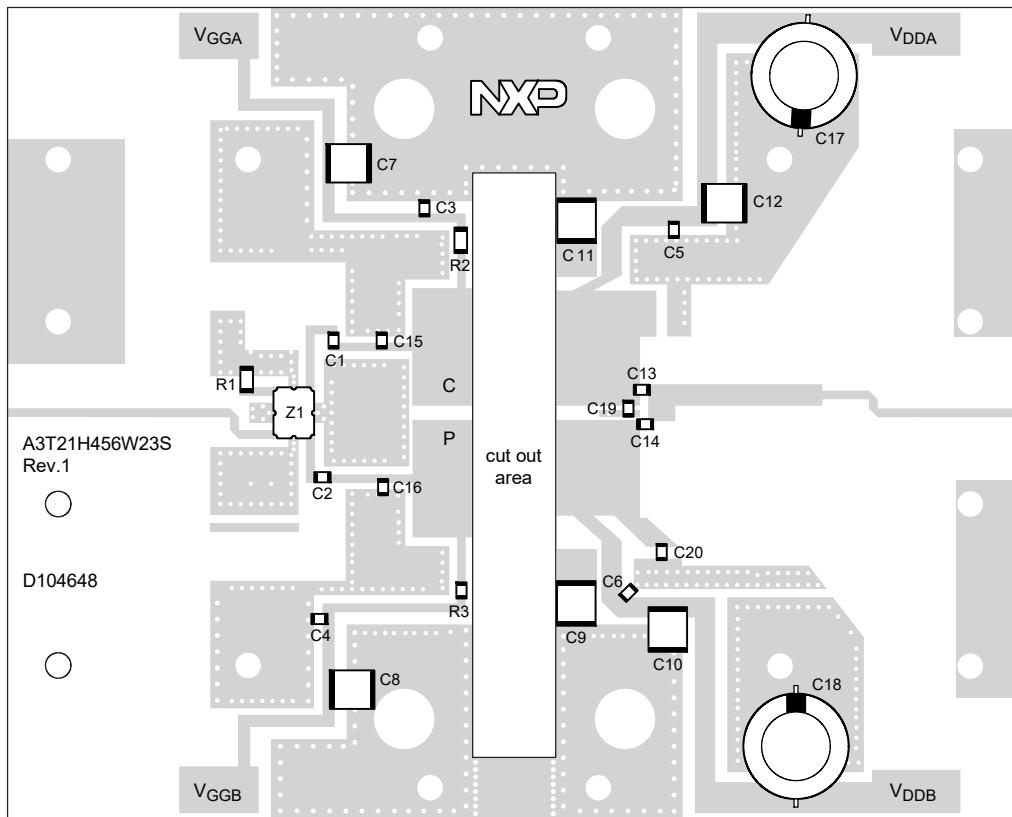
Note:  $V_{DDA}$  and  $V_{DDB}$  must be tied together and powered by a single DC power supply.
