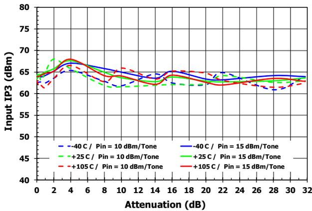
**Input IP3 vs Attenuation [3.92 GHz]**
