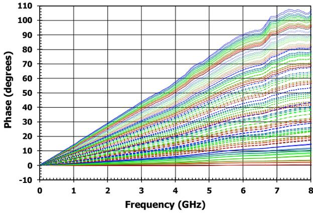
Relative Insertion Phase vs Attenuation
