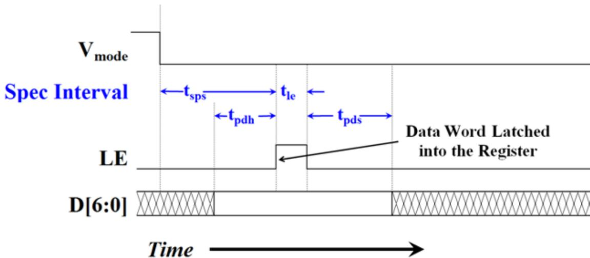
**Figure 5 - Latched Parallel Mode Timing Diagram**
