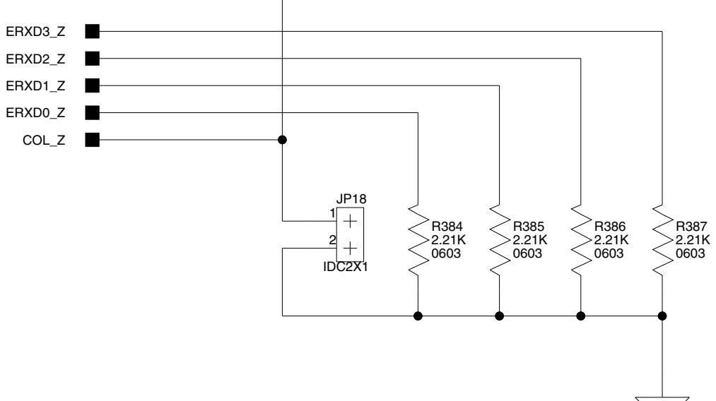
Install JP18 to put the part in Isolate mode
