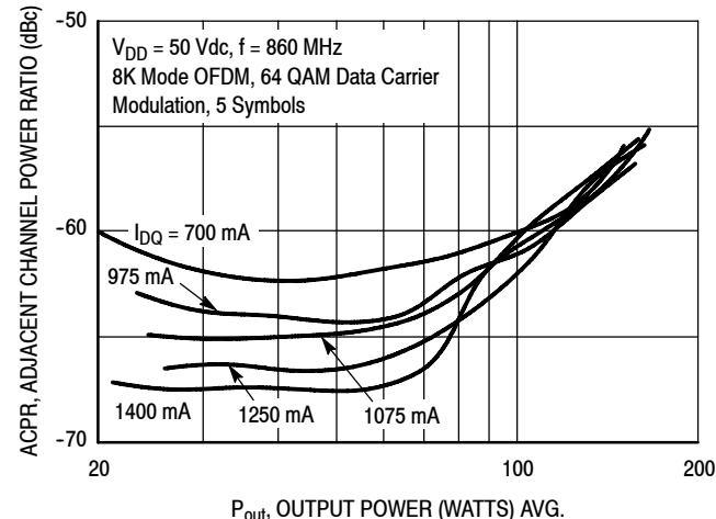
**Figure 17. Single-Carrier DVB-T OFDM ACPR versus Output Power**
