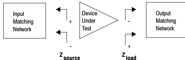
Figure 24. Series Equivalent Source and Load Impedance
