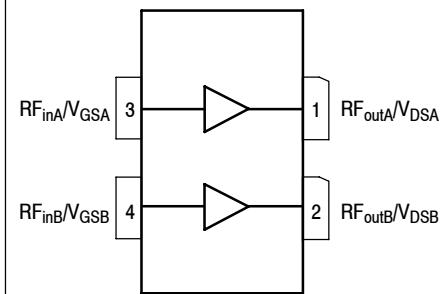
Figure 1. Pin Connections
