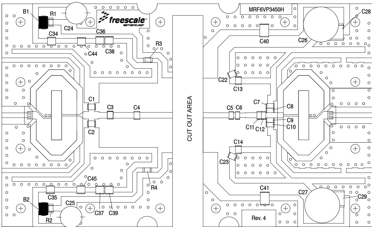
**Figure 3. MRF6VP3450HR6(HSR6) Test Circuit Component Layout — Top**
