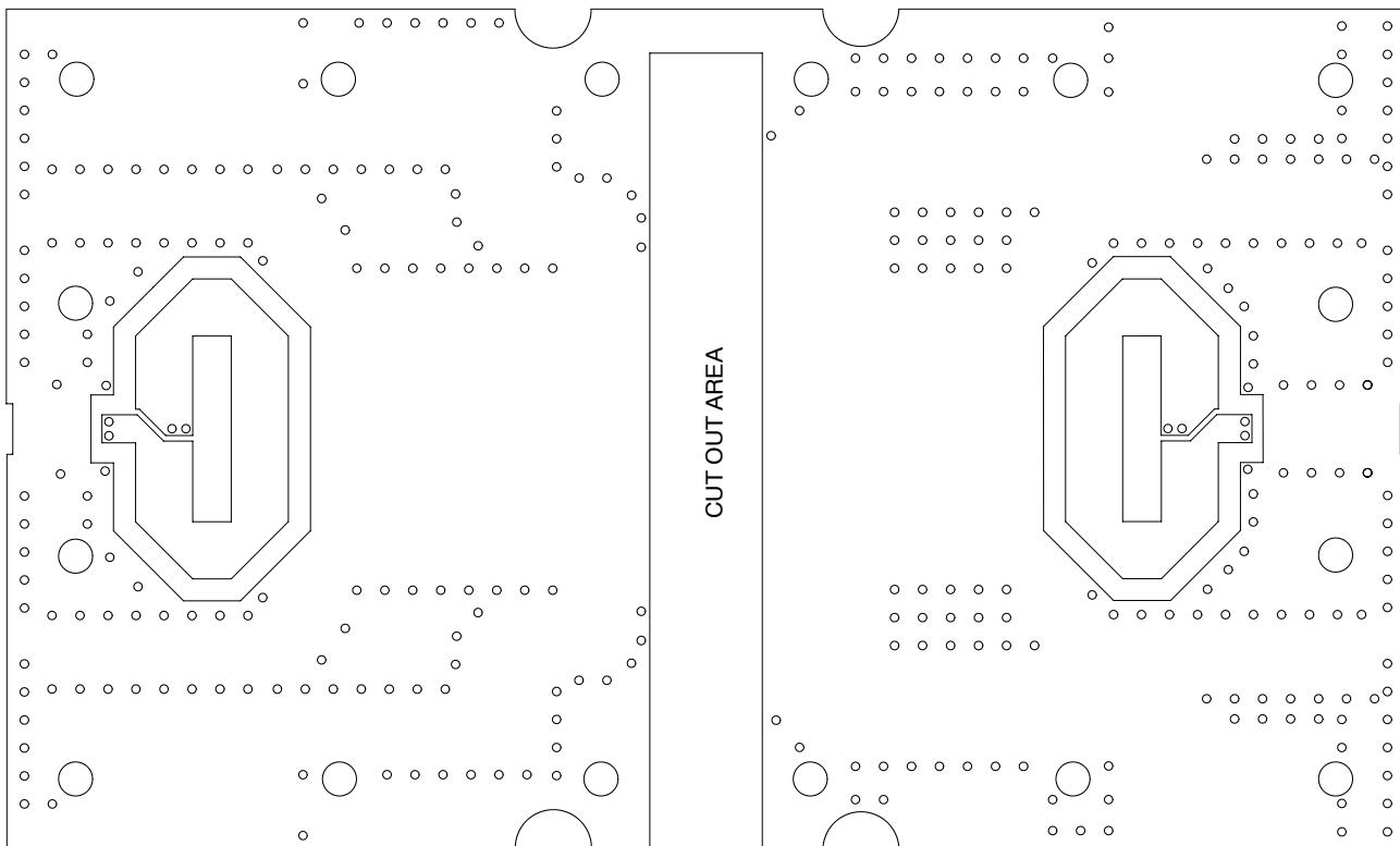
**Figure 3a. MRF6VP3450HR6(HSR6) Test Circuit Component Layout — Bottom**
