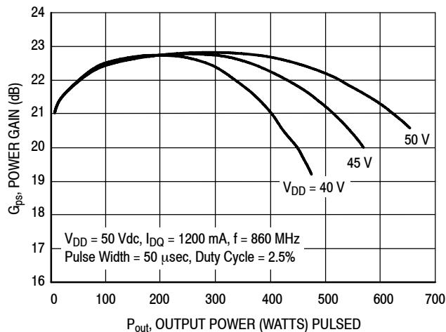
**Figure 8. Pulsed Power Gain versus Output Power**
