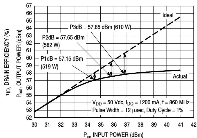
**Figure 7. Pulsed CW Output Power versus Input Power**
