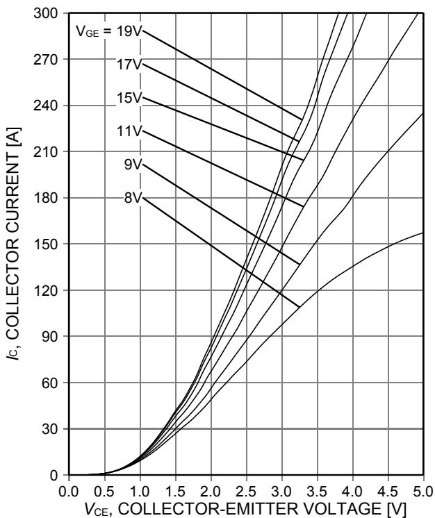
**Figure 5. Typical output characteristic**
