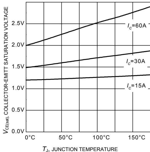
**Figure 8. Typical collector-emitter saturation voltage as a function of junction temperature**
