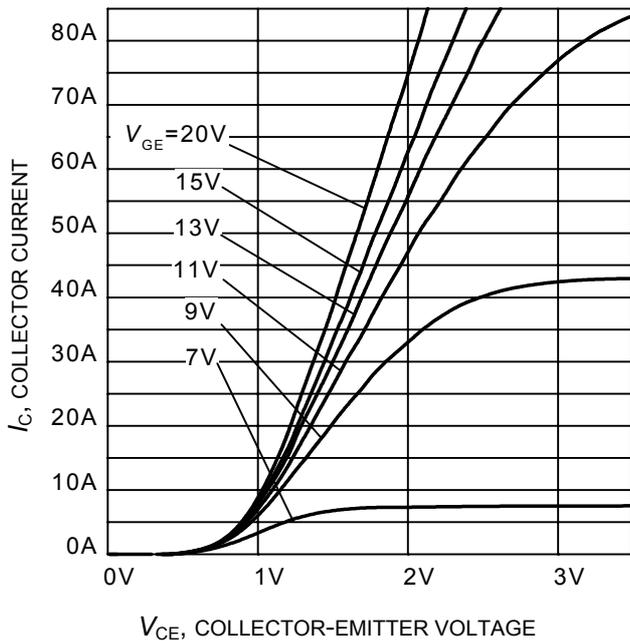
**Figure 5. Typical output characteristic**
