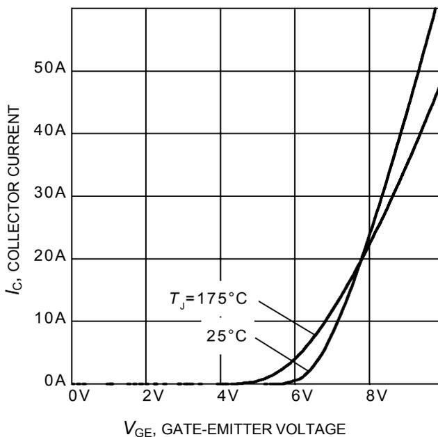
**Figure 7. Typical transfer characteristic**
