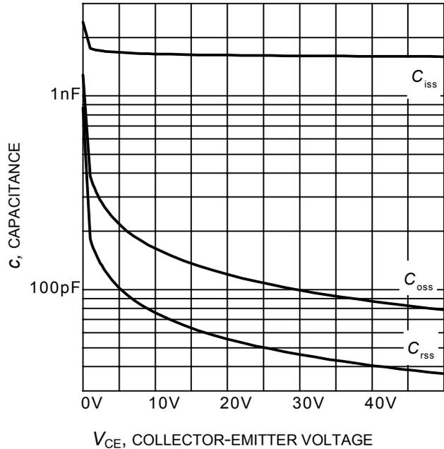
**Figure 18. Typical capacitance as a function of collector-emitter voltage**
