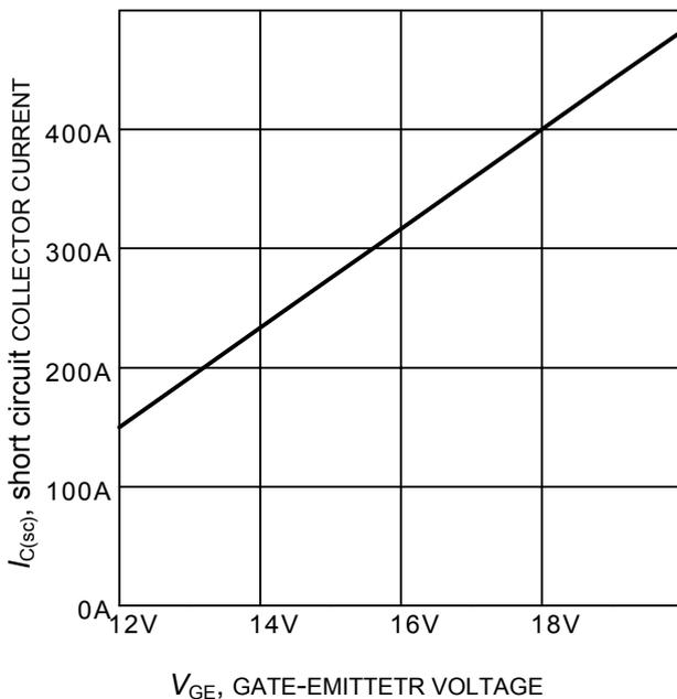
**Figure 19. Typical short circuit collector current as a function of gate-emitter voltage**
