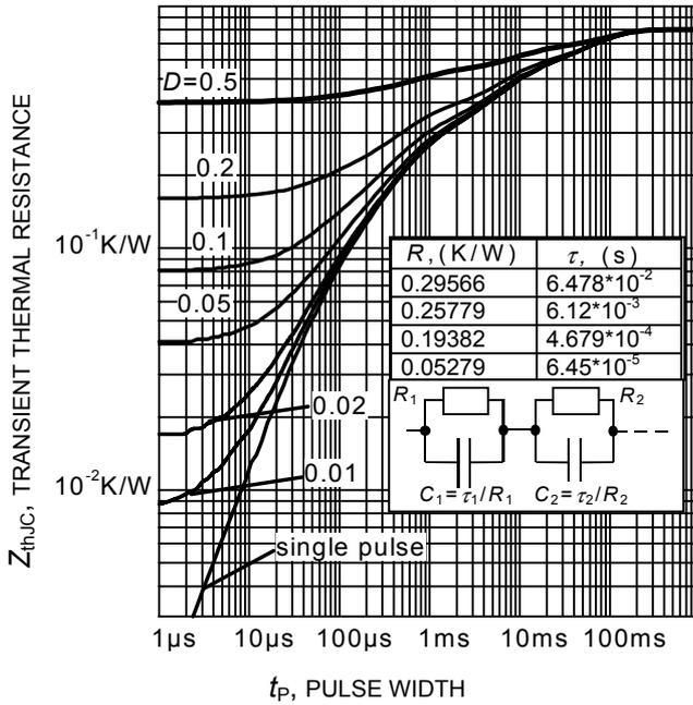
**Figure 21. IGBT transient thermal resistance**
