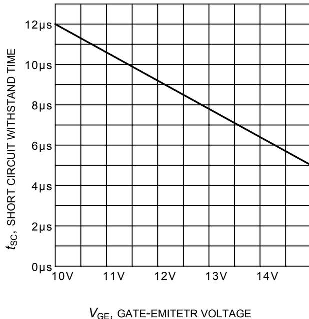
**Figure 20. Short circuit withstand time as a function of gate-emitter voltage**
