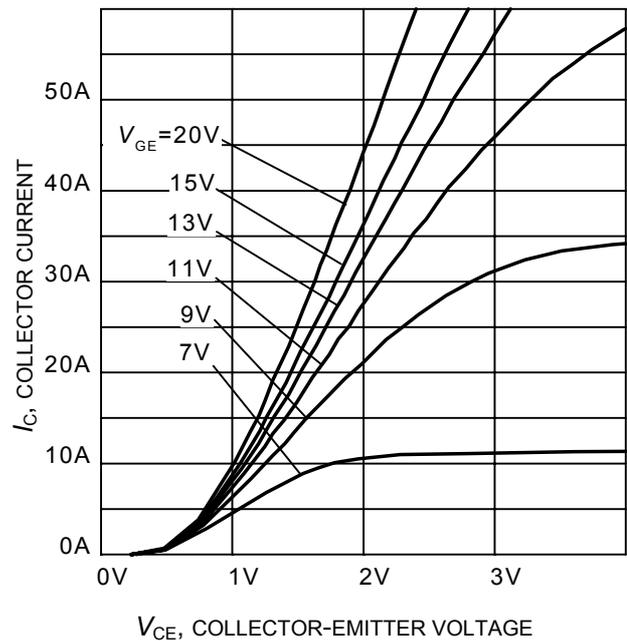
**Figure 6. Typical output characteristic**
