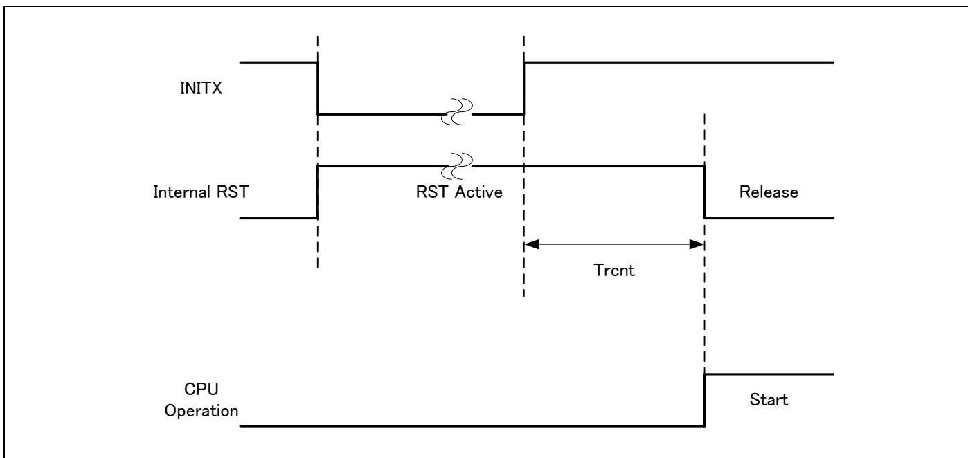
**Operation example of return from low power consumption mode (by internal resource reset\*)**
