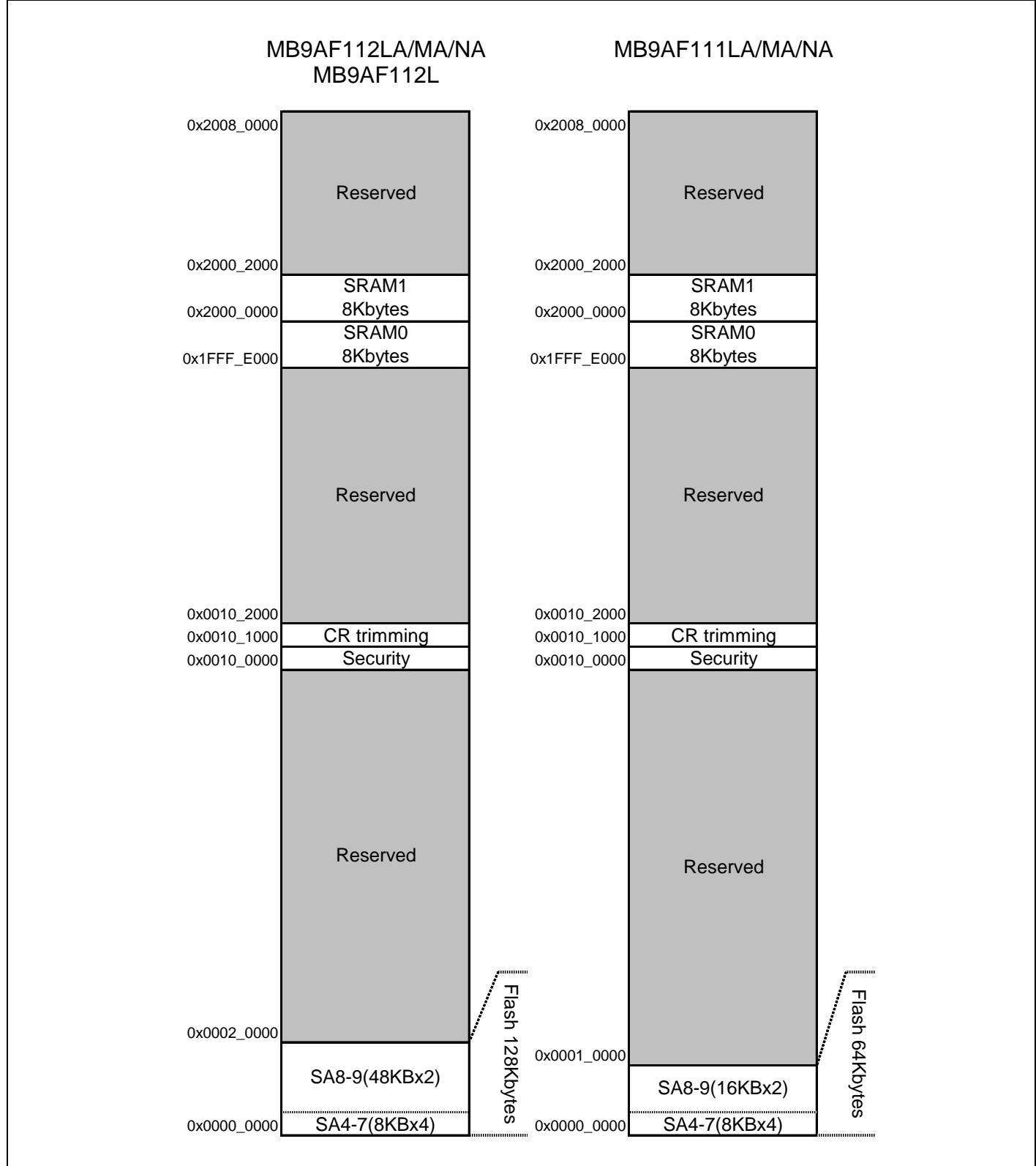
See "MB9A310A/110A Series Flash programming Manual" for sector structure of Flash.
