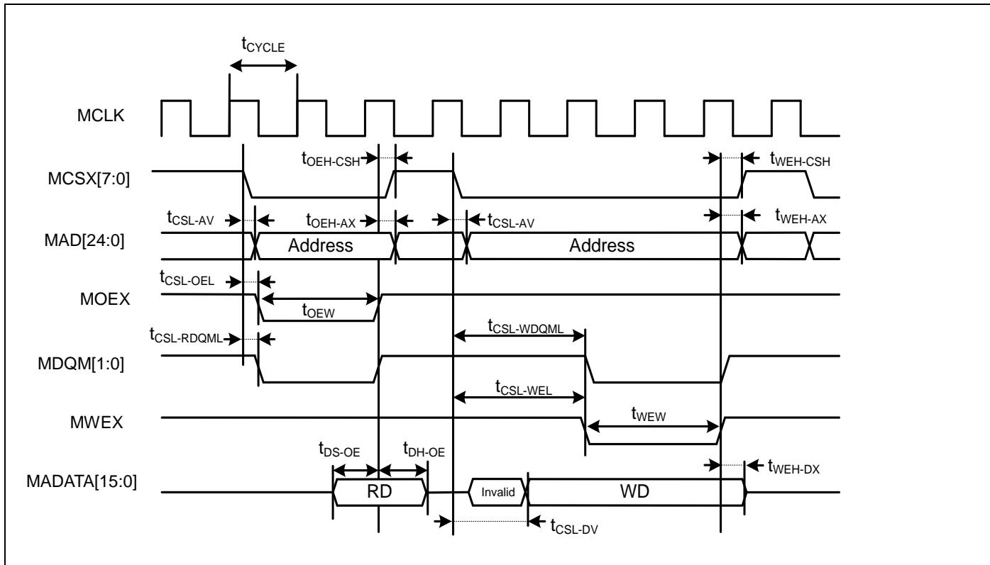
**Separate Bus Access Synchronous SRAM Mode**
