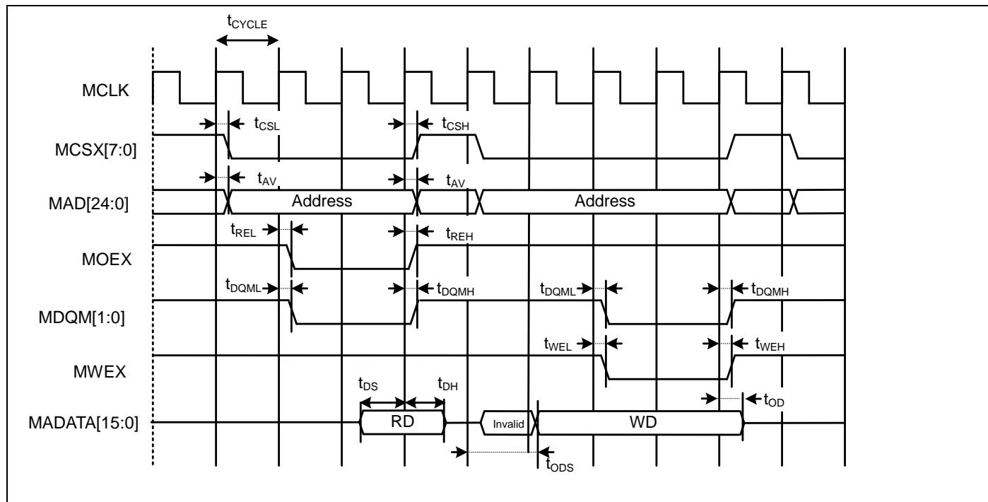
**Multiplexed Bus Access Asynchronous SRAM Mode**
