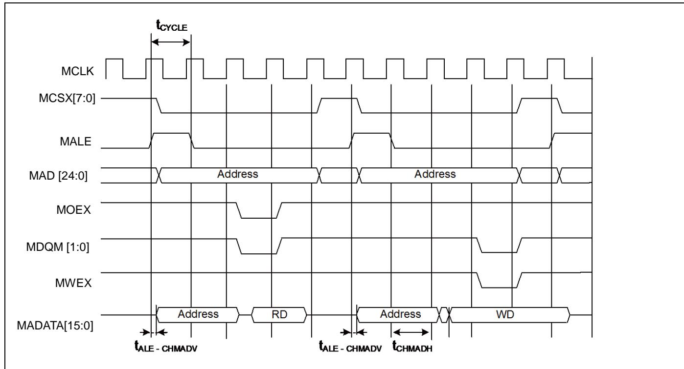
**Multiplexed Bus Access Synchronous SRAM Mode**
