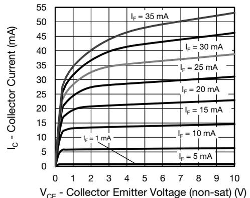
Fig. 6 - Collector Current vs. Collector Emitter Voltage
