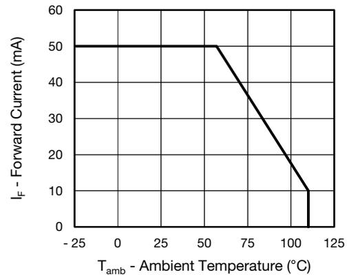
Fig. 2 - Forward Current vs. Ambient Temperature
