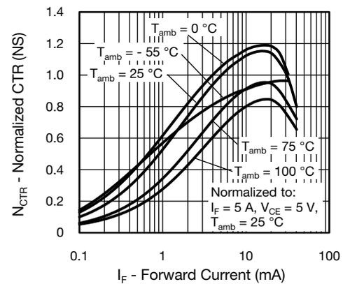
Fig. 12 - Normalized CTR (non-saturated) vs. Forward Current
