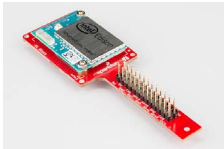
Headers on Edison side
