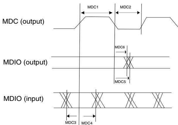
**Figure 29. MII/RMII serial management channel timing diagram**
