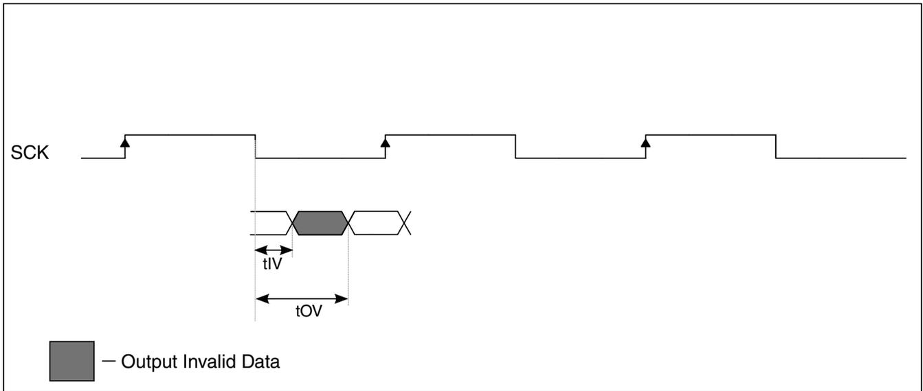
Figure 13. QuadSPI output timing (HyperRAM mode) diagram
