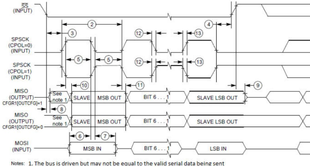
**Figure 22. LPSPI slave mode timing (CPHA = 1)**
