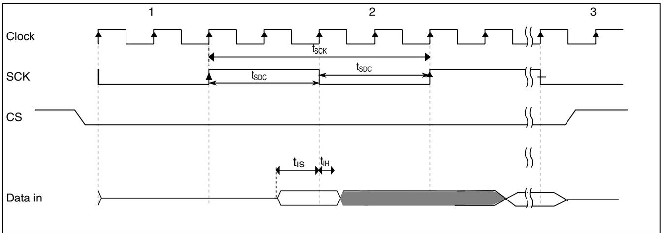
Figure 10. QuadSPI input timing (SDR mode) diagram
