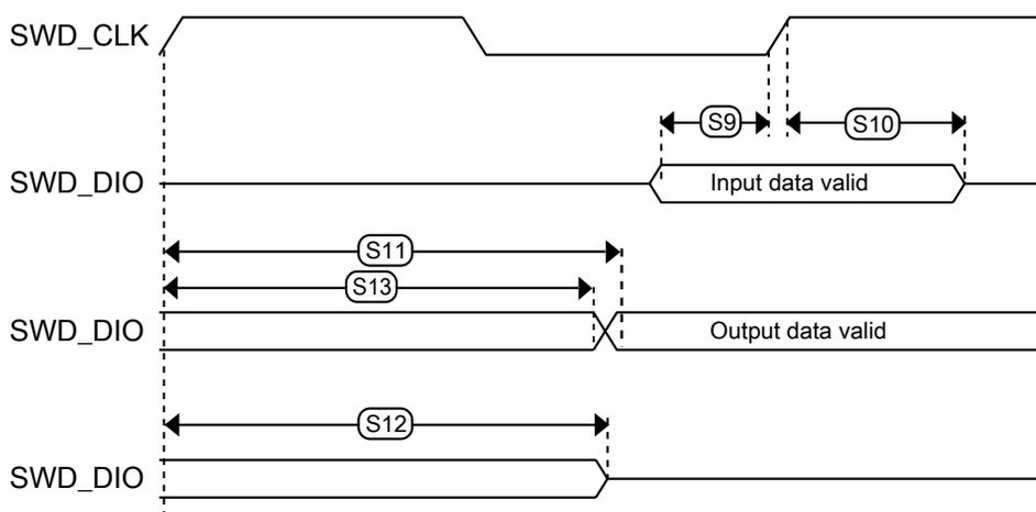
Figure 31. Serial wire data timing
