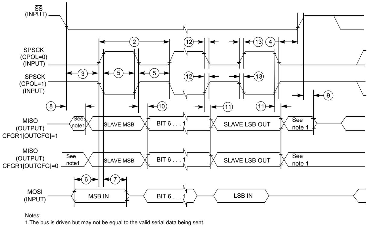
**Figure 21. LPSPI slave mode timing (CPHA = 0)**
