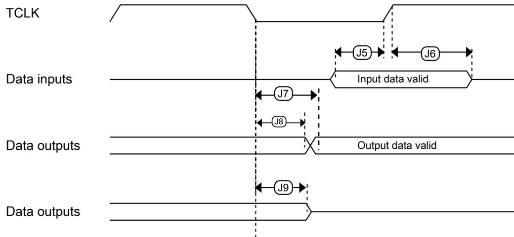
**Figure 34. Boundary scan (JTAG) timing**
