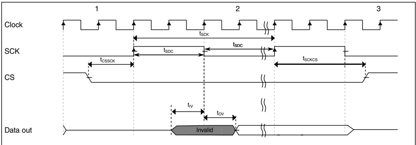
Figure 11. QuadSPI output timing (SDR mode) diagram
