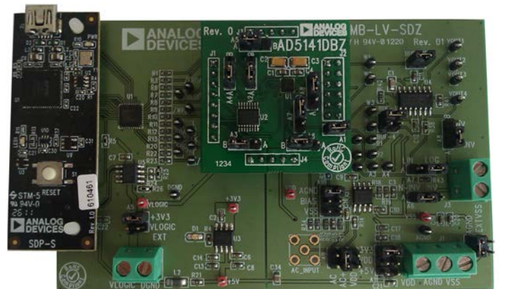
Figure 1. Digital Picture of Evaluation Board with Low Voltage DigiPOT Motherboard and System Demonstration Platform
