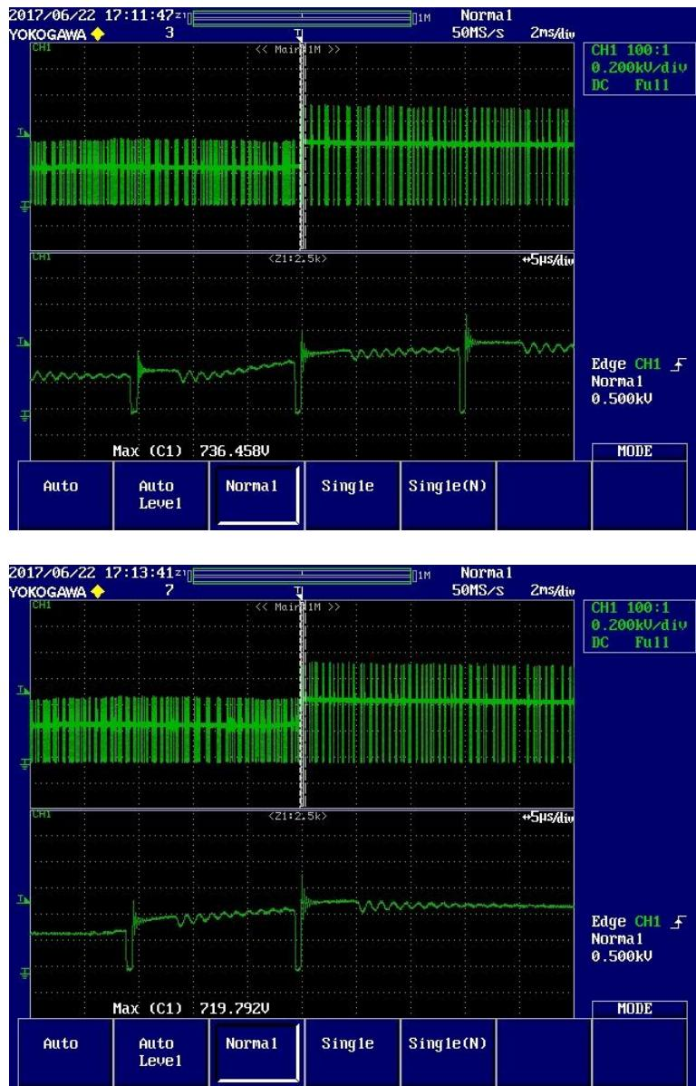
**Figure 58 – Differential Mode Surge Test at 500 V.**
