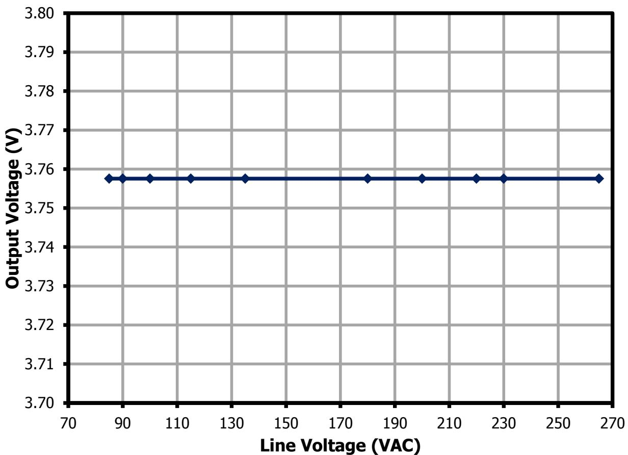
**Figure 13 – 3.8 V Output Voltage vs. Input Line Voltage, Room Temperature.**
