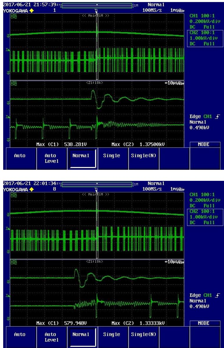
**Figure 59 – Ring Wave Surge Test at 2.5 kV.**
