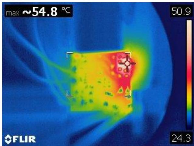
**Figure 17** – Measured Temperature at 0.3 W,
