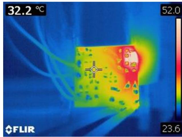
**Figure 19** – Measured Temperature at 0.3 W,
