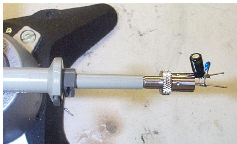
**Figure 46** – Oscilloscope Probe with Probe Master ([www.probemaster.com](http://www.probemaster.com)) 4987A BNC Adapter. (Modified with wires for ripple measurement, and two parallel decoupling capacitors added)
