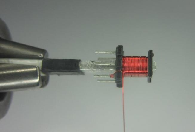
A photograph showing the completed winding. The red wire has been wound 123 turns in four layers and is now secured at the top-left terminal (pin 1) with black tape.            | Finish at pin 1.                                                                                                                                                        |
