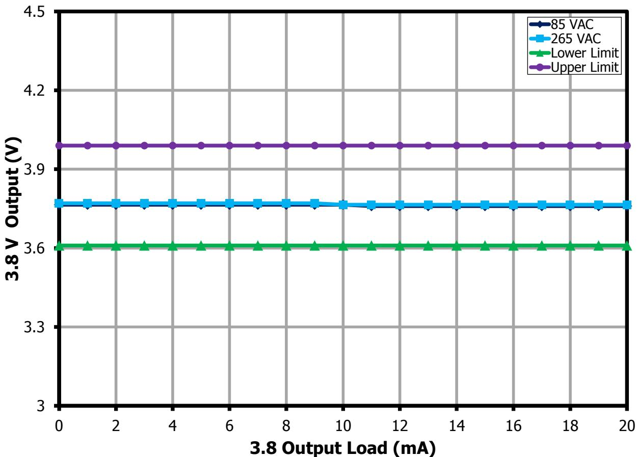
**Figure 14 – 3.8 V Output Voltage with Varying Load.**
