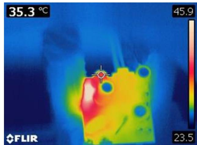
**Figure 16** – Measured Temperature at 0.3 W,
