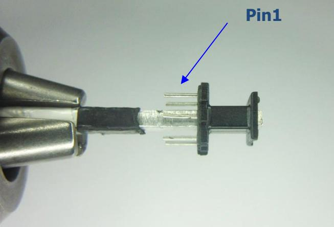
A photograph of a transformer bobbin mounted on a winder. A blue arrow points to the top-left terminal, labeled "Pin1".                                                            | For the purpose of these instructions, bobbin is oriented on winder such that pin side is on the left side (see illustration). Winding direction as shown is clockwise. |
