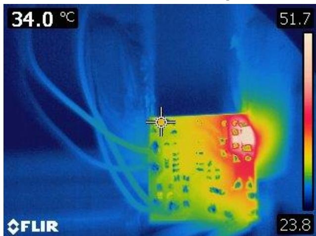
**Figure 15** – Measured Temperature at 0.3 W,
