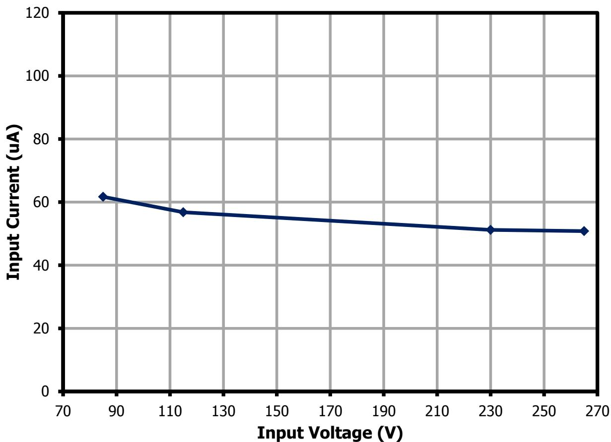
**Figure 11** – Input Current at Standby vs. Input Line Voltage, Room Temperature.
