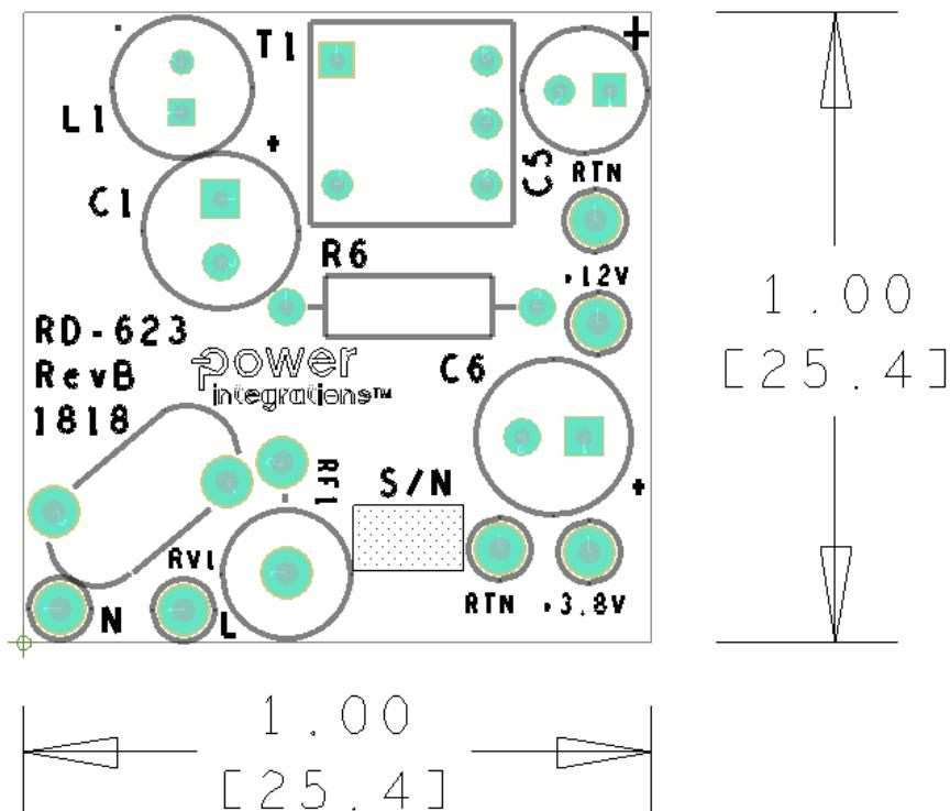
**Figure 4** – Printed Circuit Layout, Top.
