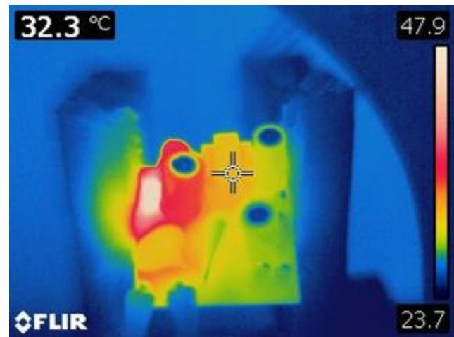
**Figure 18** – Measured Temperature at 0.3 W,
