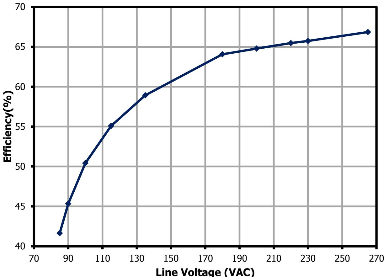
**Figure 8 – Efficiency vs. Line Voltage, Room Temperature.**
