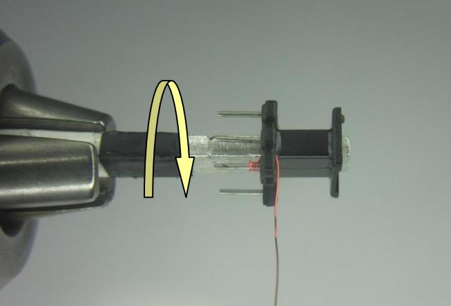
A photograph showing the initial winding step. A yellow arrow indicates the direction of winding starting from the bottom terminal (pin 3) towards the top-left terminal (pin 1). | Starting at pin 3, wind 123 turns of wire Item [4] in four layers.                                                                                                      |
