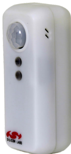
Figure 1.1. Zigbee Occupancy Sensor Reference Design
