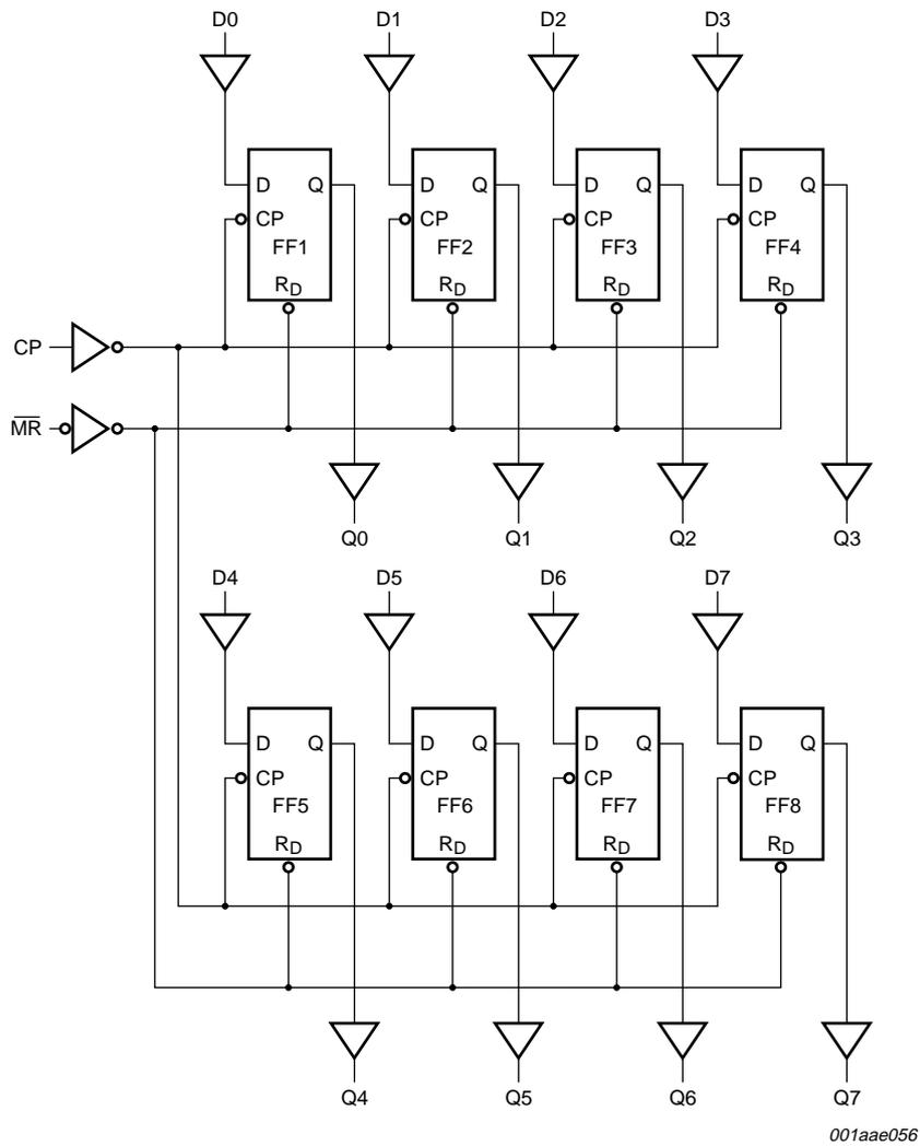
Fig 3. Logic diagram
