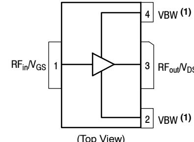
**Figure 1. Pin Connections**
