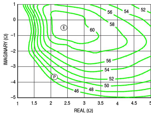
Figure 9. P1dB Load Pull Efficiency Contours (%)
