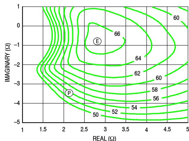
Figure 13. P3dB Load Pull Efficiency Contours (%)
