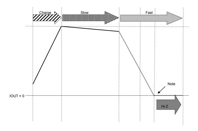
Note: When the motor current reaches zero level (Iout = 0 A), the output becomes "Hi-Z" state.
