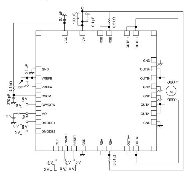
Note: The addition of a bypass capacitor is recommended if necessary. The GND wiring should be connected to one point as much as possible.
