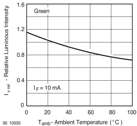
Figure 16. Rel. Luminous Intensity vs. Ambient Temperature
