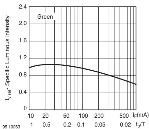
Figure 17. Specific Luminous Intensity vs. Forward Current
