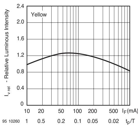
Figure 12. Rel. Lumin. Intensity vs. Forw. Current/Duty Cycle
