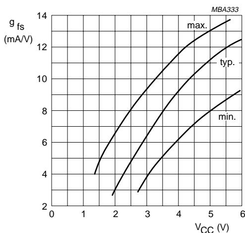
Fig.12 Typical forward transconductance  $g_{fs}$  as a function of the supply voltage at  $V_{CC}$  at  $T_{amb} = 25^\circ C$ .
