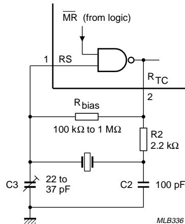
Fig.15 External components configuration for a crystal oscillator.
