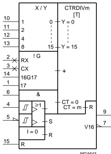
Fig.2 IEC logic diagram.
