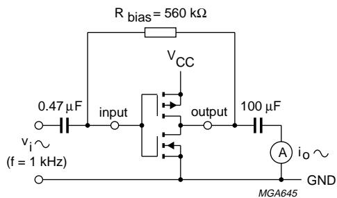
Fig.11 Test set-up for measuring forward transconductance  $g_{fs} = di_o/dv_i$  at  $v_o$  is constant (see Fig.12) and MR = LOW.
