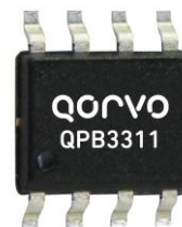
Package: SOIC-8 with Exposed Pad
