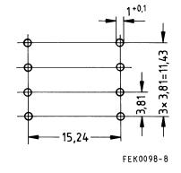
Hole arrangement View in mounting direction
