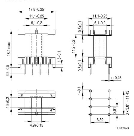
Hole arrangement View in mounting direction
