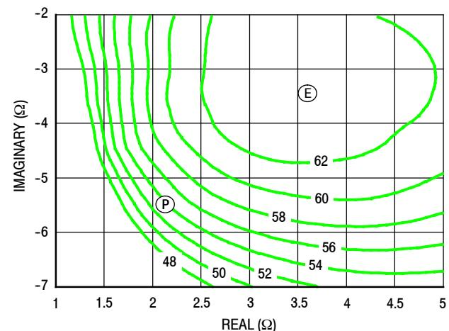
Figure 23. P1dB Load Pull Efficiency Contours (%)
