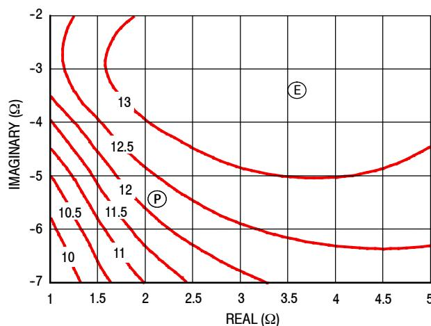
Figure 24. P1dB Load Pull Gain Contours (dB)
