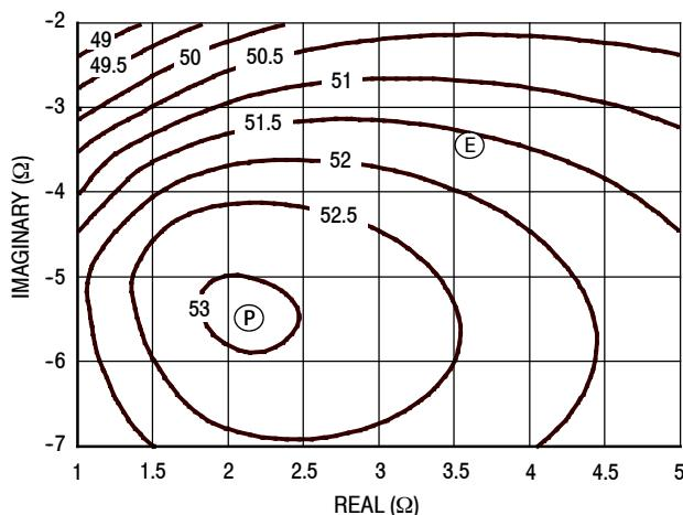
Figure 22. P1dB Load Pull Output Power Contours (dBm)
