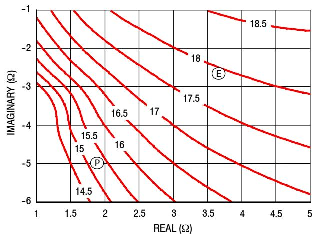
Figure 20. P3dB Load Pull Gain Contours (dB)
