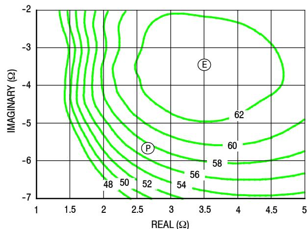
Figure 27. P3dB Load Pull Efficiency Contours (%)
