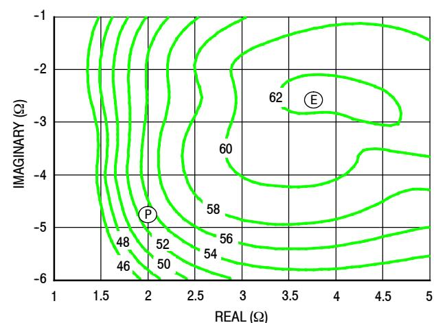
Figure 15. P1dB Load Pull Efficiency Contours (%)
