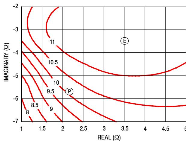
Figure 28. P3dB Load Pull Gain Contours (dB)
