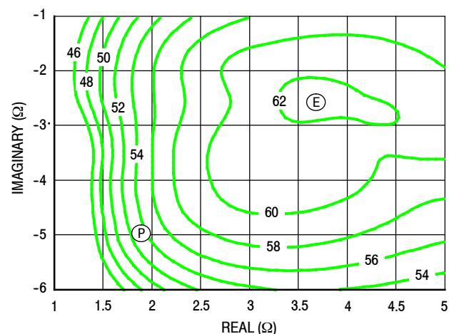
Figure 19. P3dB Load Pull Efficiency Contours (%)
