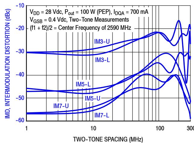
Figure 5. Intermodulation Distortion Products versus Two-Tone Spacing — AFT26H250W03S
