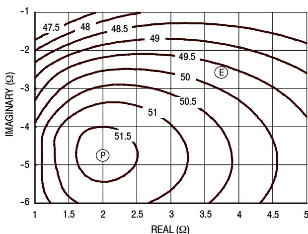
Figure 14. P1dB Load Pull Output Power Contours (dBm)
