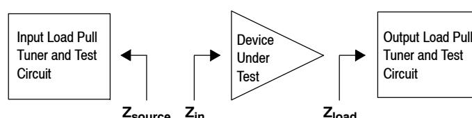
$V_{DD} = 28$  Vdc,  $V_{GSB} = 0.4$  mA, Pulsed CW, 10  $\mu$ sec(on), 10% Duty Cycle
