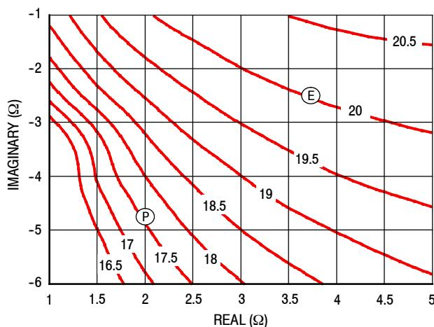
Figure 16. P1dB Load Pull Gain Contours (dB)
