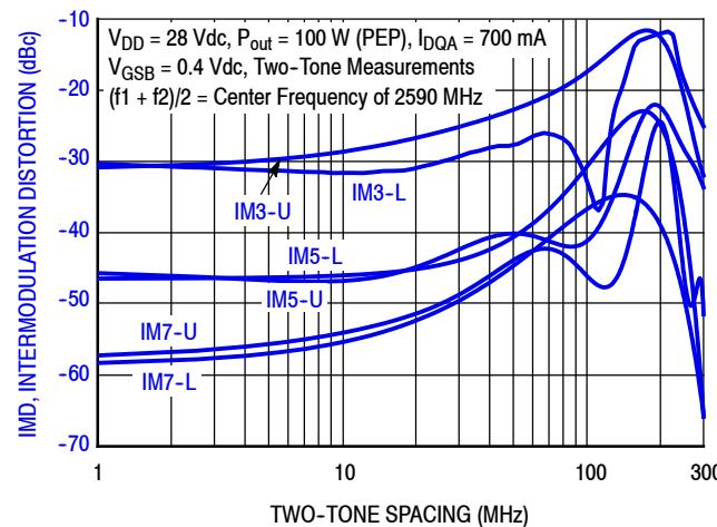
Figure 6. Intermodulation Distortion Products versus Two-Tone Spacing — AFT26H250-24S
