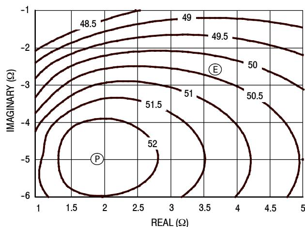
Figure 18. P3dB Load Pull Output Power Contours (dBm)
