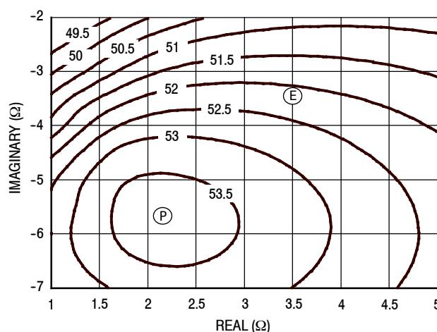
Figure 26. P3dB Load Pull Output Power Contours (dBm)
