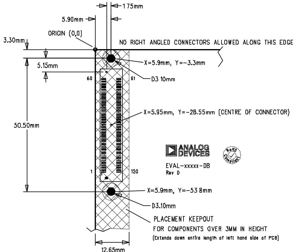
Figure 2-4. Connector Placement on Compatible Daughter Board
