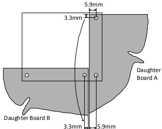
Figure 2-3. Maximum Board Dimensions for Connector Placement
