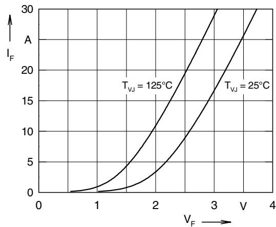
Fig. 20 Typ. forward characteristics of free wheeling diode
