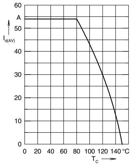
Fig. 5 Max. forward current versus case temperature
