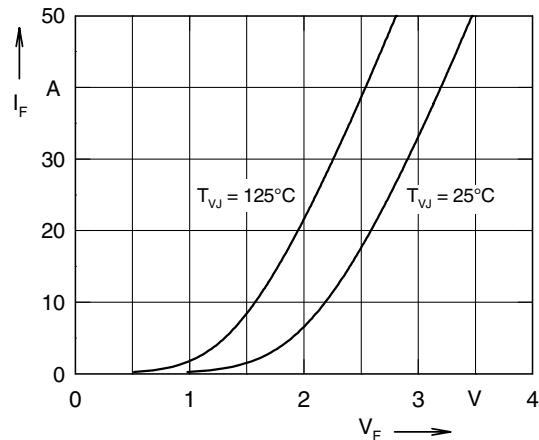
Fig. 10 Typ. forward characteristics of free wheeling diode
