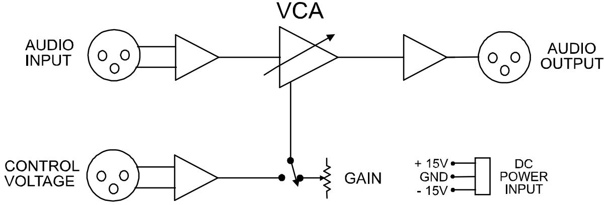
Figure 1. 2180-DEMO Block Diagram
