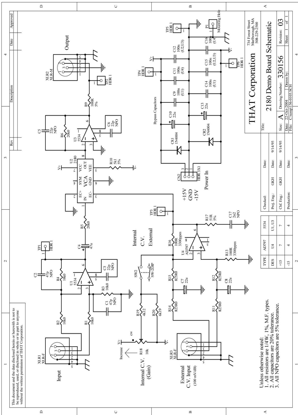
Figure 3. 2180-DEMO Schematic
