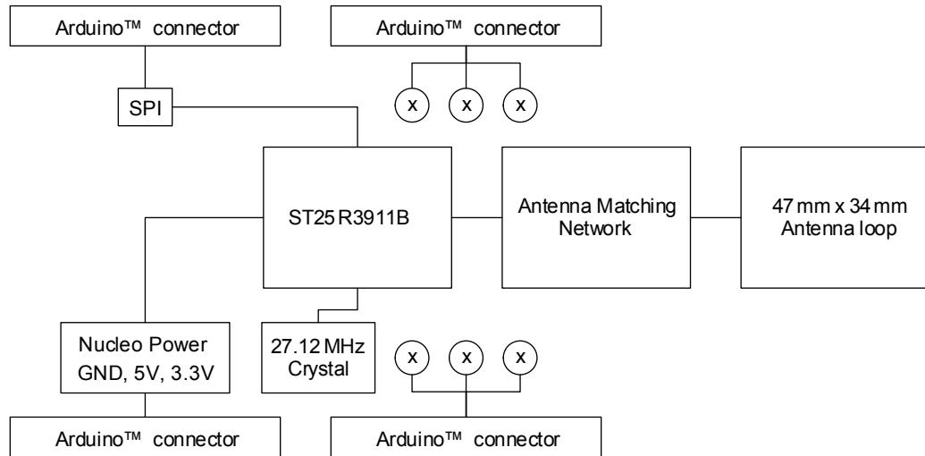
**Figure 2. X-NUCLEO-NFC05A1 evaluation board circuit schematic (1 of 3)**
