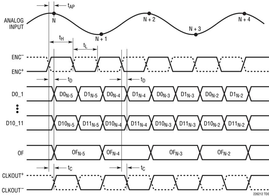
**Double Data Rate LVDS Output Mode Timing**
