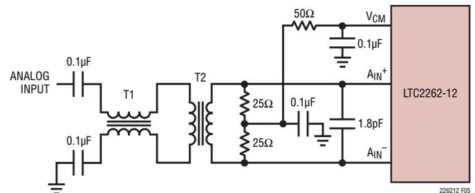
**Figure 5. Recommended Front-End Circuit for Input Frequencies from 170MHz to 270MHz**
