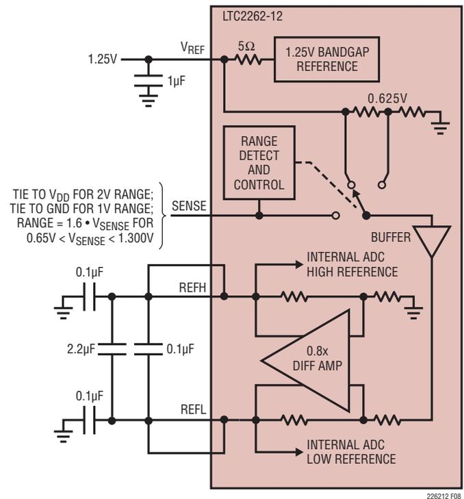
Figure 8. Reference Circuit
