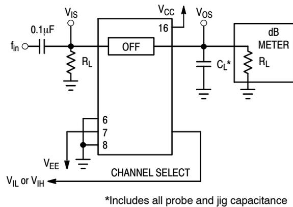
**Figure 13. Off Channel Feedthrough Isolation, Test Set-Up**
