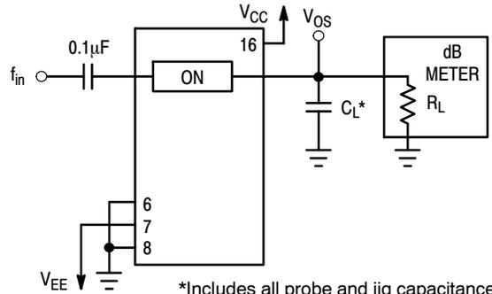
**Figure 12. Maximum On Channel Bandwidth, Test Set-Up**
