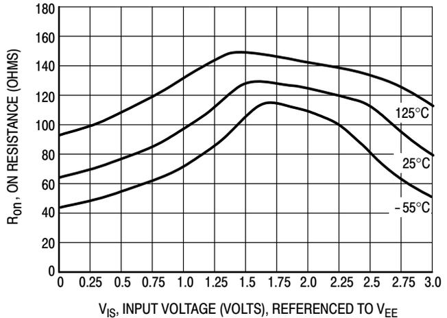
Figure 7b. Typical On Resistance, V<sub>CC</sub> - V<sub>EE</sub> = 3.0 V
