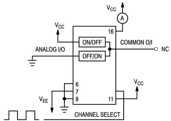
**Figure 19. Power Dissipation Capacitance, Test Set-Up**
