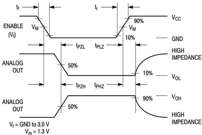
**Figure 17a. Propagation Delays, Enable to Analog Out**
