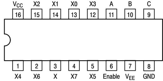
**Figure 2. Pinout: MC74HCT4051A**
