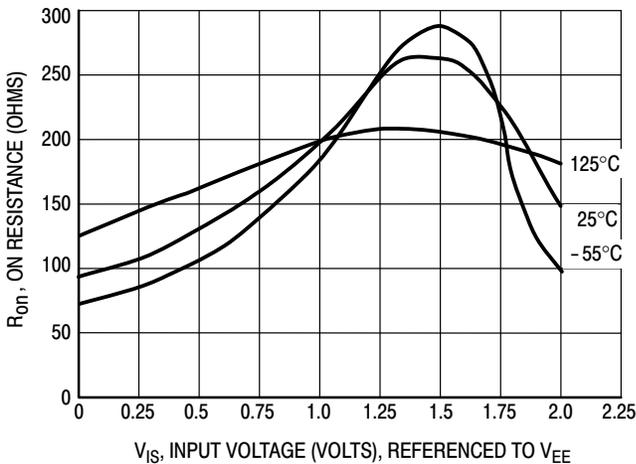
Figure 7a. Typical On Resistance, V<sub>CC</sub> - V<sub>EE</sub> = 2.0 V
