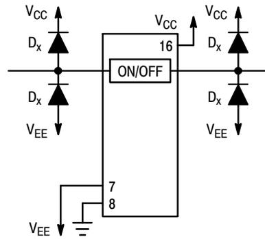
Figure 22. External Germanium or Schottky Clipping Diodes
