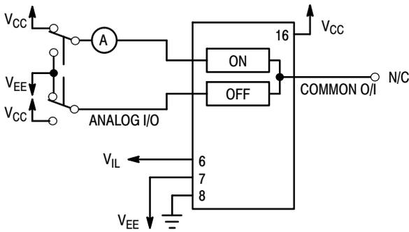
**Figure 11. Maximum On Channel Leakage Current, Channel to Channel, Test Set-Up**
