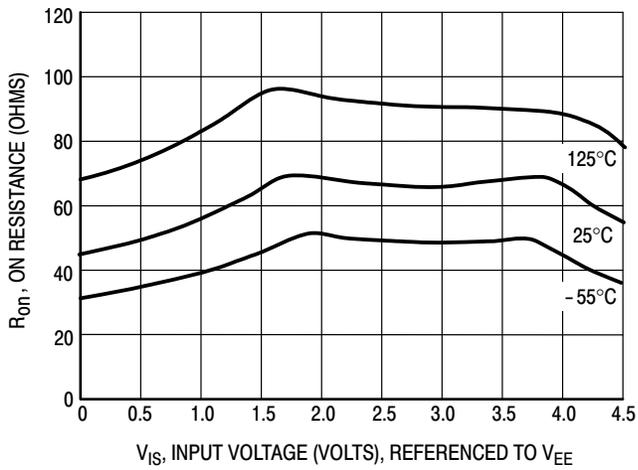
Figure 7c. Typical On Resistance,  $V_{CC} - V_{EE} = 4.5 \text{ V}$
