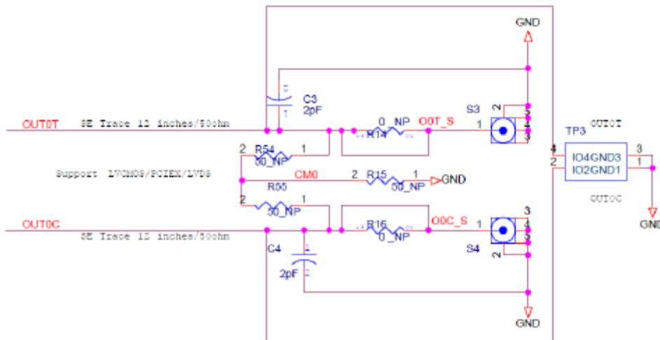
The circuit is designed for maximum flexibility when testing all possible logic types. Default assembly uses a 0.1μF capacitor in place of R14 and R16, and the short across R14 and R16 is cut. No other devices are assembled. This simple AC-coupled configuration allows for testing phase noise and jitter of all possible logic types. The circuit can be modified for custom tests. TP3 is a position to place a differential FET probe.
