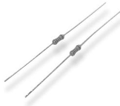
The resistive element comprises a thin film of nickel-chrome alloy evaporated onto a high thermal conductivity ceramic element. Metal end caps are force fitted to the element prior to spiralling to value. Tinned copper lead wires are welded to the end caps and the components are then coated. One coat of phenolic resin is followed by three coats of epoxy resin. All resistors are tested for value and tolerance.
