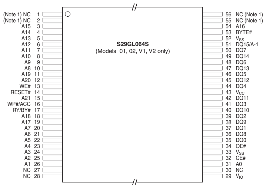
Figure 2. 56-Pin Standard TSOP
