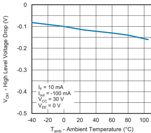
Fig. 10 - High Level Voltage Drop vs. Ambient Temperature
