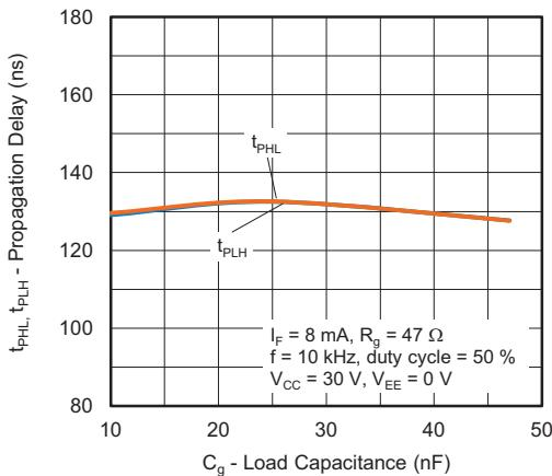
Fig. 16 - Propagation Delay vs. Load Capacitance
