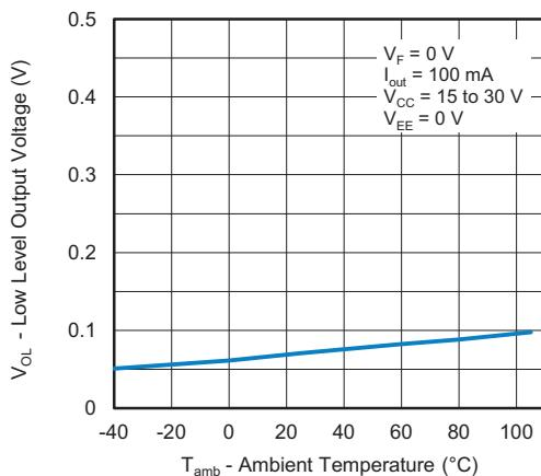
Fig. 9 - Low Level Output Voltage vs. Ambient Temperature
