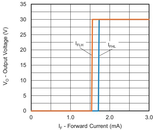
Fig. 6 - Output Voltage vs. Forward Current
