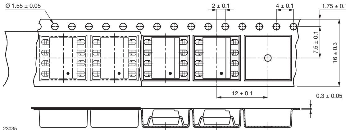
Fig. 24 - Tape and Reel Packaging (1000 pieces on reel)
