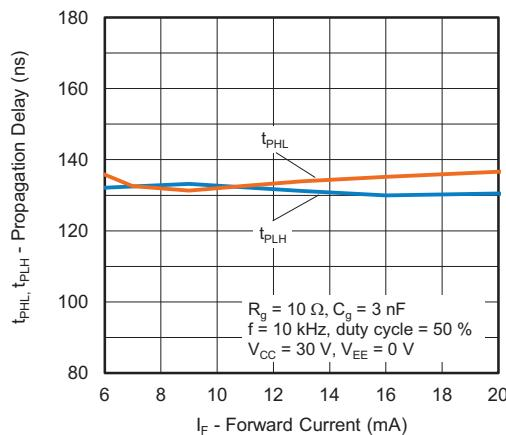
Fig. 12 - Propagation Delay vs. Forward Current
