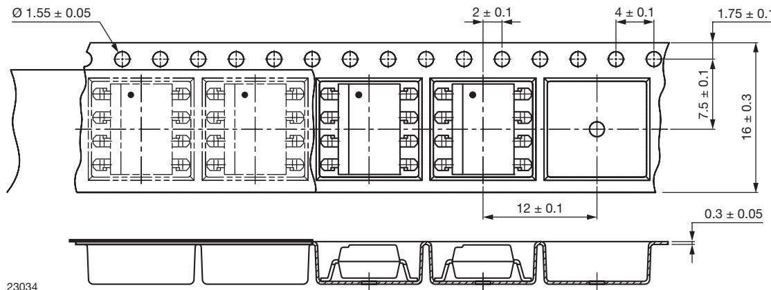
Fig. 23 - Tape and Reel Packaging (1000 pieces on reel)
