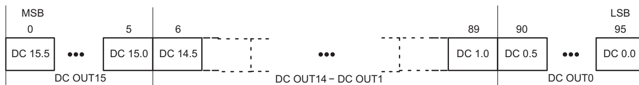
Figure 15. Dot Correction Data Packet Format
