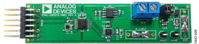
Figure 9. EVAL-CN0370-PMDZ Circuit Evaluation Board
