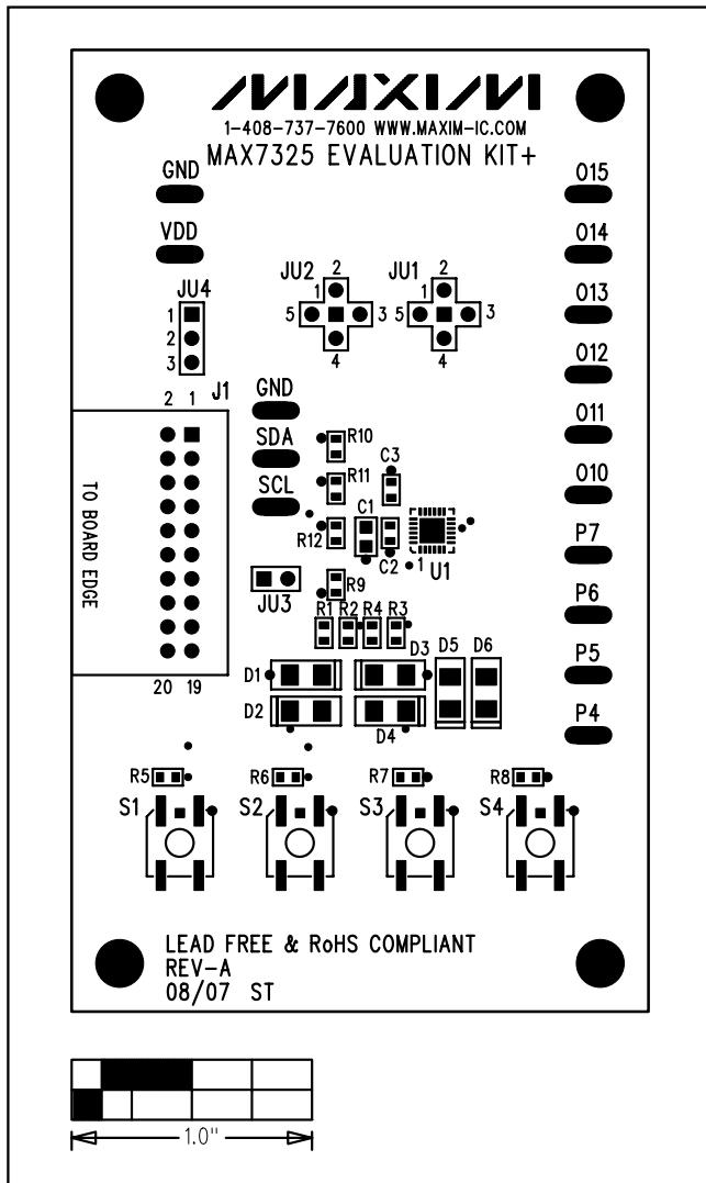
Figure 3. MAX7325 EV Kit Component Placement Guide—Component Side
