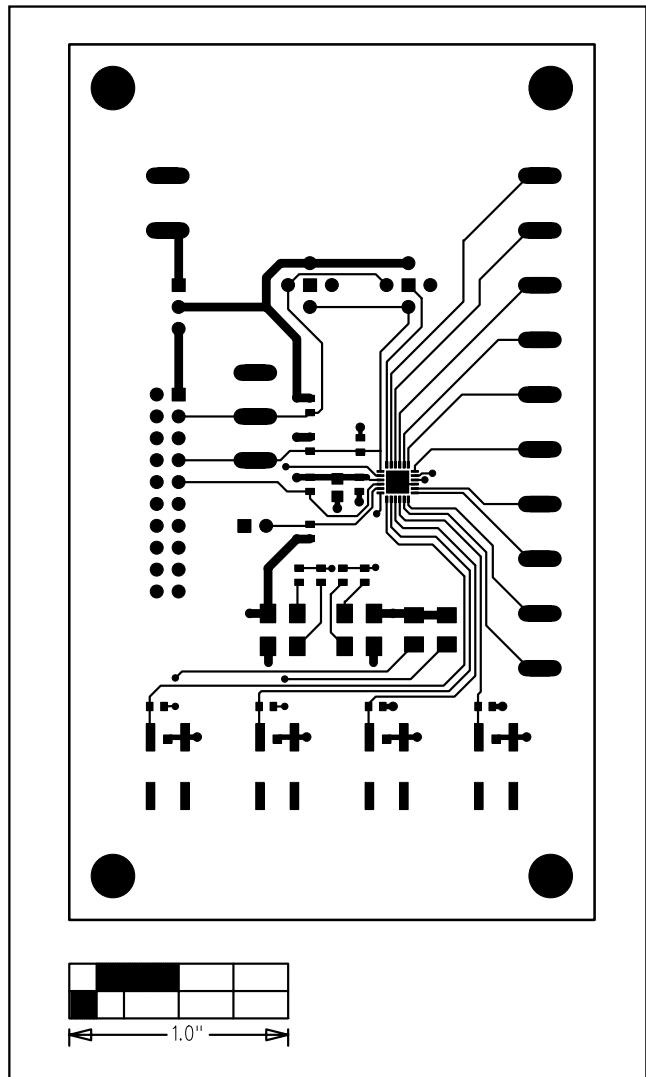
Figure 4. MAX7325 EV Kit PCB Layout—Component Side
