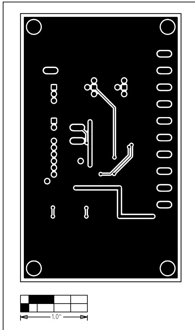
Figure 5. MAX7325 EV Kit PCB Layout—Solder Side
