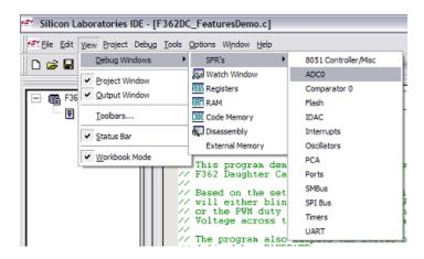
2. In the debug window, change the value of **ADC0CN** from 0x82 to 0x02. This value turns off the ADC on the target microcontroller.
