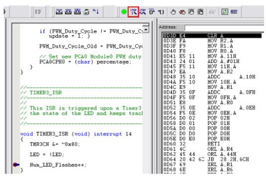
The disassembly window has three columns. The left column is the address of the instruction in Flash. The middle column is the instruction in hex. The right column is the disassembled instruction. The Disassembly debug window and the capability to single-step through firmware allows a developer to see exactly what instructions are executed and their output.
