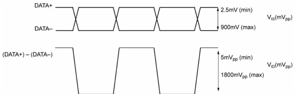
Figure 1.  $V_{IS}$  and  $V_{ID}$  Definitions
