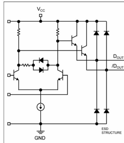
Figure 3. Output Structure
