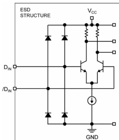
Figure 2. Input Structure
