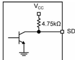
Figure 4. SD Output Structure
