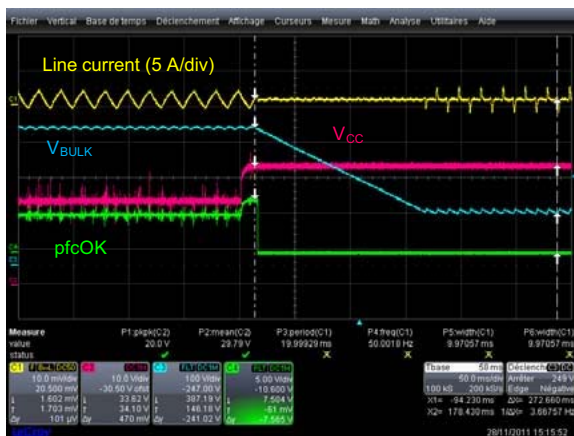
a) pfcOK being pulled-up above 7.5 V, the part latches off
