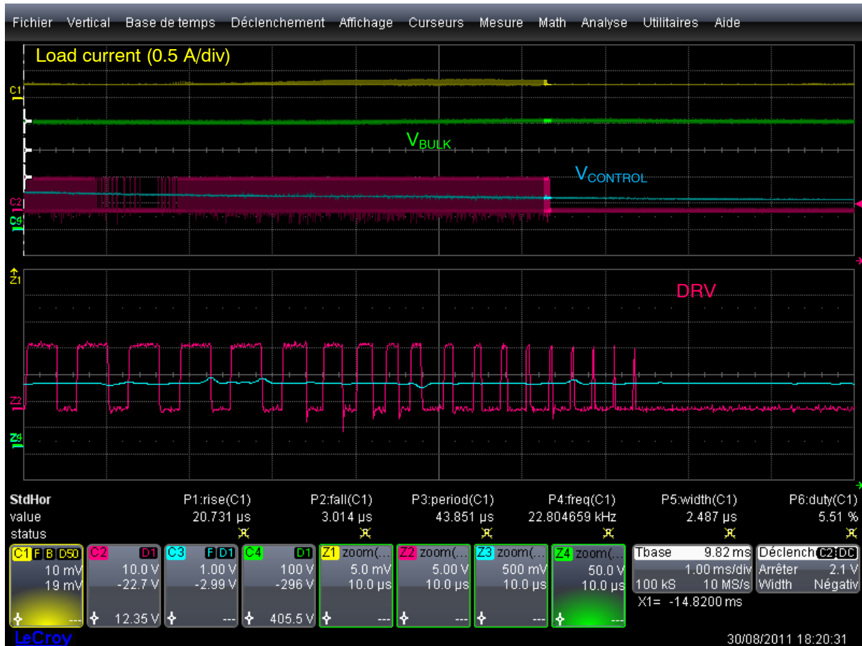
Figure 16. Soft Over-Voltage Protection
