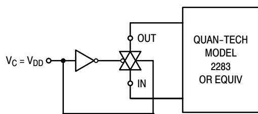
**Figure 9. Noise Voltage Test Circuit**
