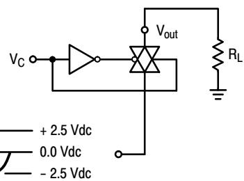
**Figure 12. Frequency Response Test Circuit**
