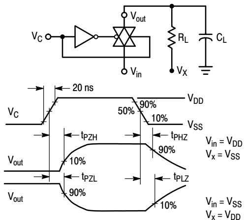
**Figure 7. Turn-On Delay Time Test Circuit and Waveforms**
