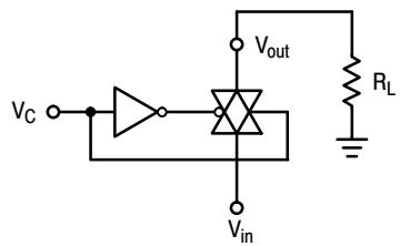
**Figure 5.  $R_{ON}$  Characteristics Test Circuit**
