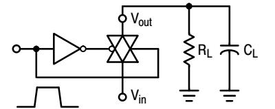
**Figure 6. Propagation Delay Test Circuit and Waveforms**
