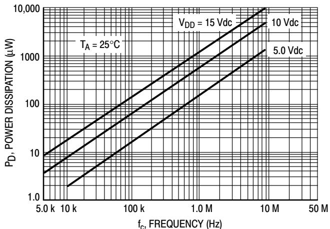
Figure 3. Typical Power Dissipation per Circuit
