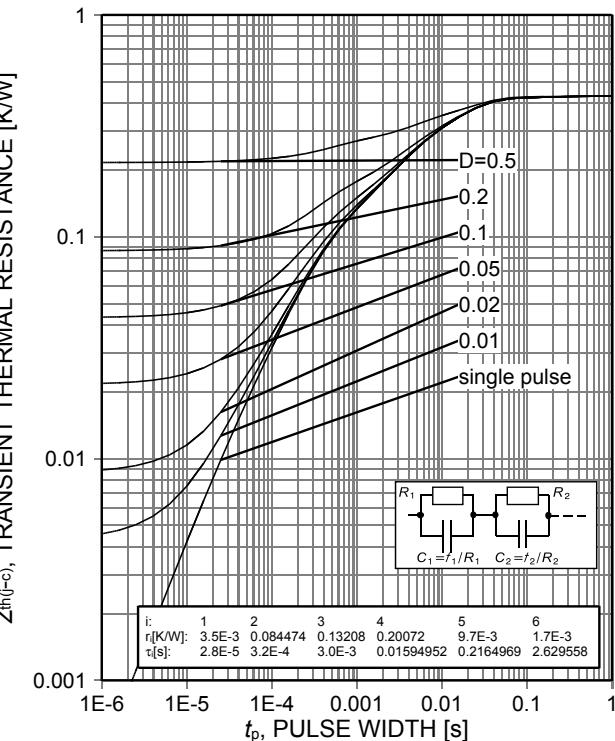
Figure 20. Diode transient thermal impedance as a
