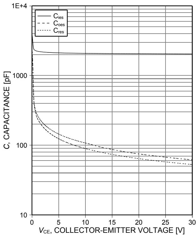
Figure 18. Typical capacitance as a function of
