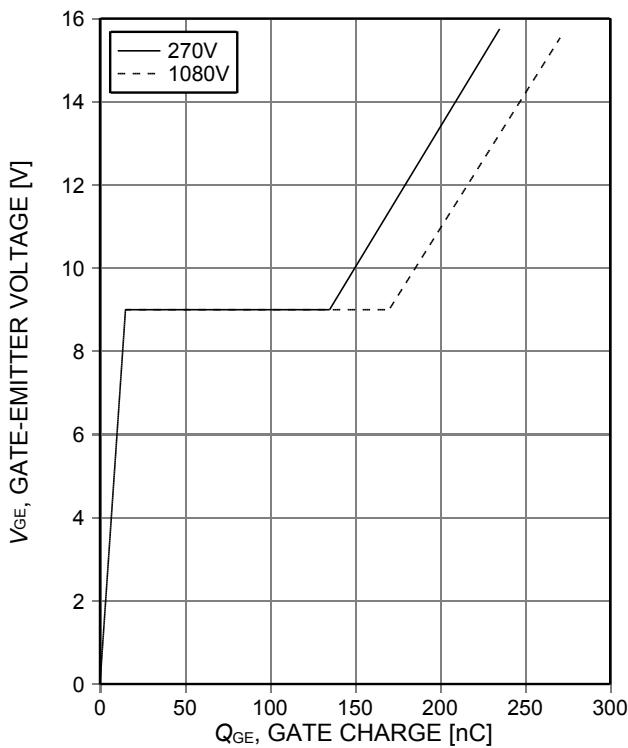
Figure 17. Typical gate charge
