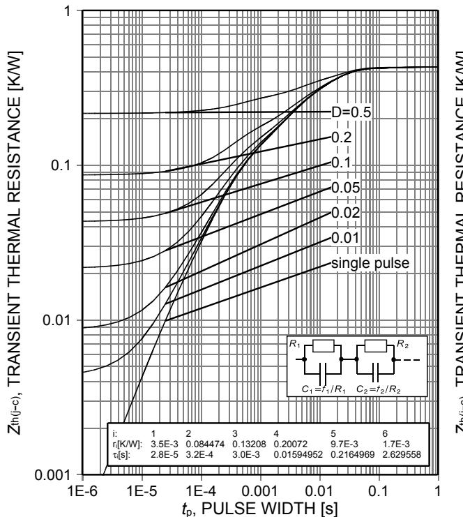
Figure 19. IGBT transient thermal resistance
