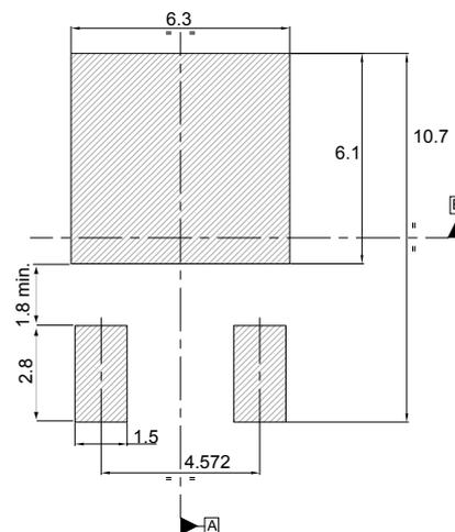
The device must be positioned within  $\oplus 0.05 \text{ A B}$
