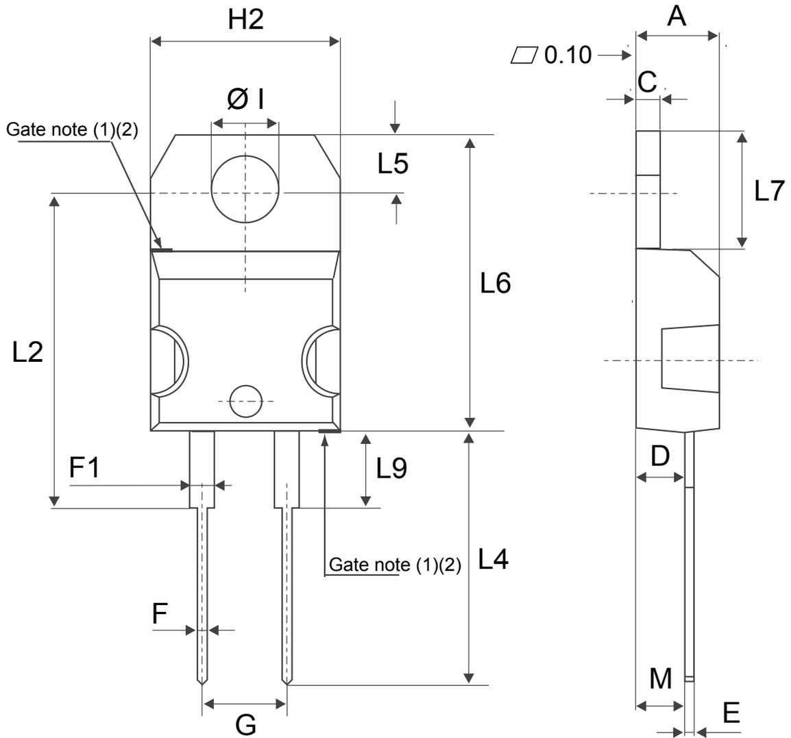
(1) :Max resin gate protusion 0.5 mm
