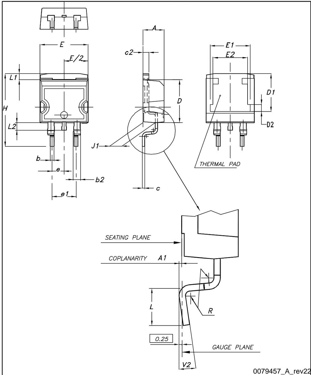
Table 10: D<sup>2</sup>PAK (TO-263) type A package mechanical data
