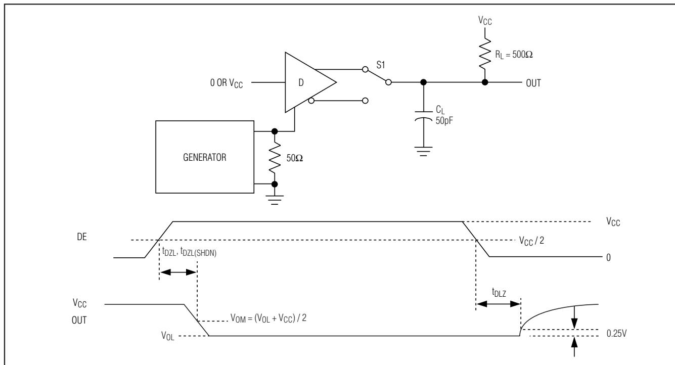
Figure 5. Driver Enable and Disable Times ( $t_{DZL}$ ,  $t_{DLZ}$ ,  $t_{DZH(SHDN)}$ )
