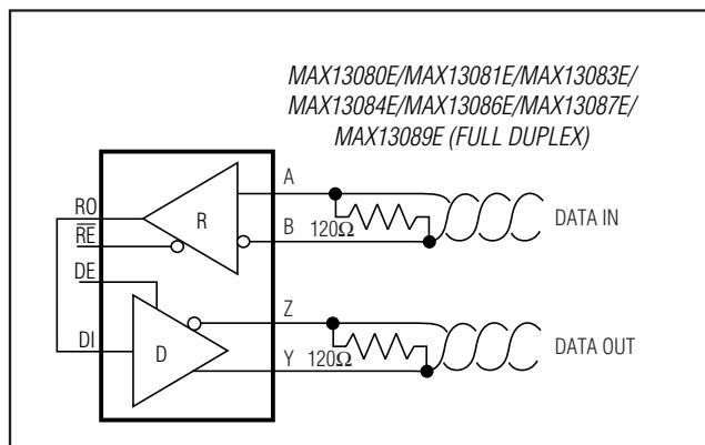
Figure 11. Line Repeater for MAX13080E/MAX13081E/MAX13083E/MAX13084E/MAX13086E/MAX13087E/MAX13089E in Full-Duplex Mode
