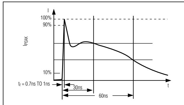
Figure 10d. IEC 61000-4-2 ESD Generator Current Waveform
