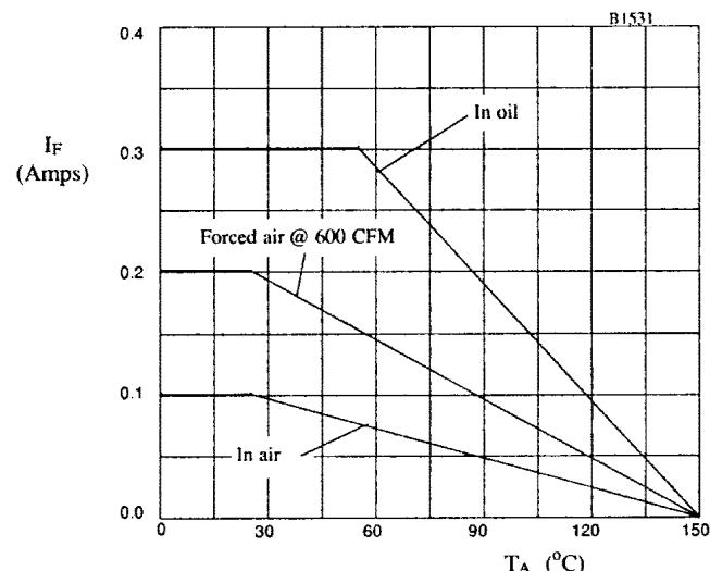
Fig 2. Maximum average forward current against ambient temperature.
