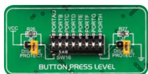
Figure 6-5: Button press level DIP switch (tri-state)
