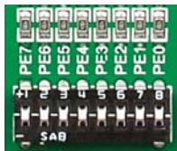
Figure 6-2: Tri-state DIP switch on PORTE
