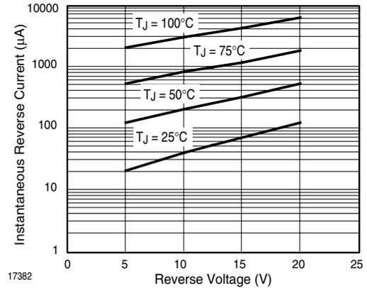
Figure 4. Typical Reverse Current Characteristics - SL02
