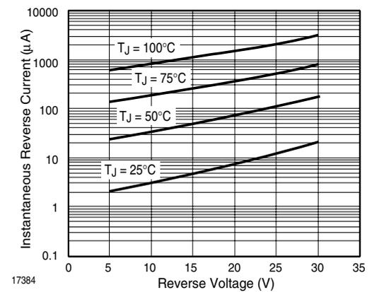
Figure 6. Typical Reverse Current Characteristics - SL03
