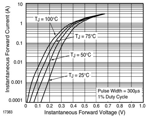
Figure 5. Typical Instantaneous Forward Characteristics - SL03
