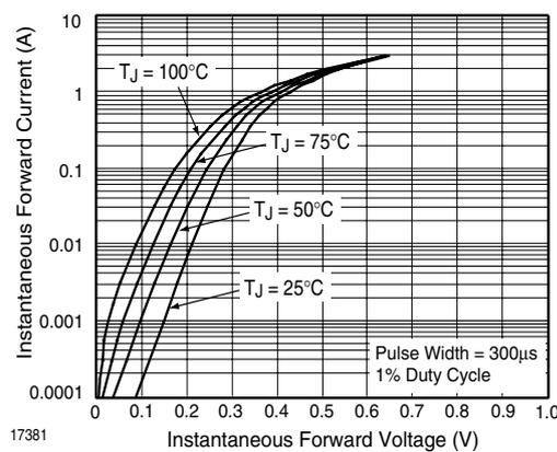
Figure 3. Typical Instantaneous Forward Characteristics - SL02
