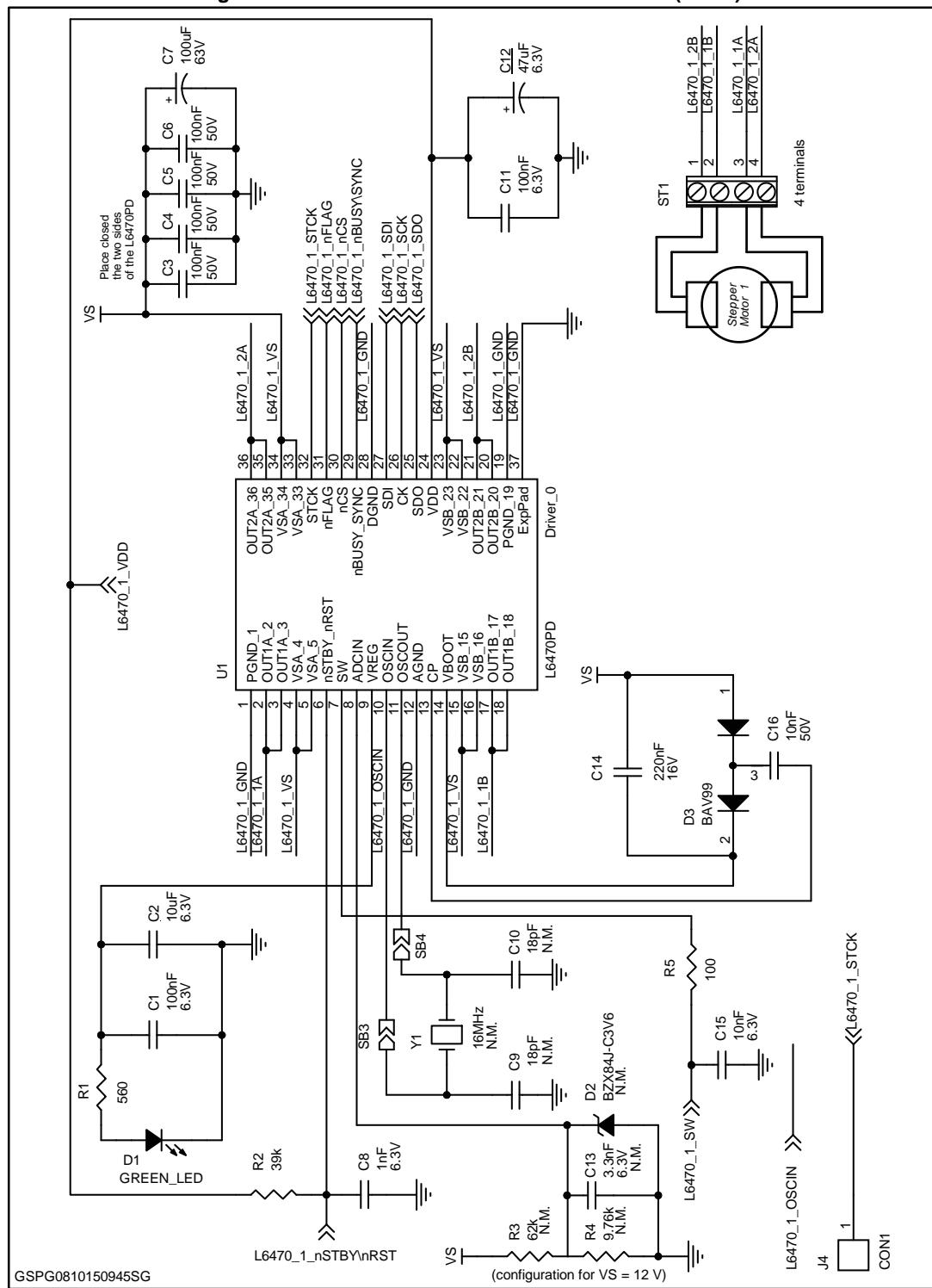
Figure 3: X-NUCLEO-IHM02A1 circuit schematic (3 of 4)
