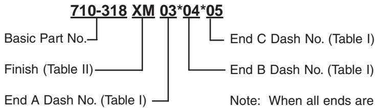
Note: When all ends are identical, insert only one dash no. When multiple dash numbers are ordered, transition size will be determined by the largest. Adapter may be supplied on smaller entries. Letter to follow entry will be supplied with adapters.
