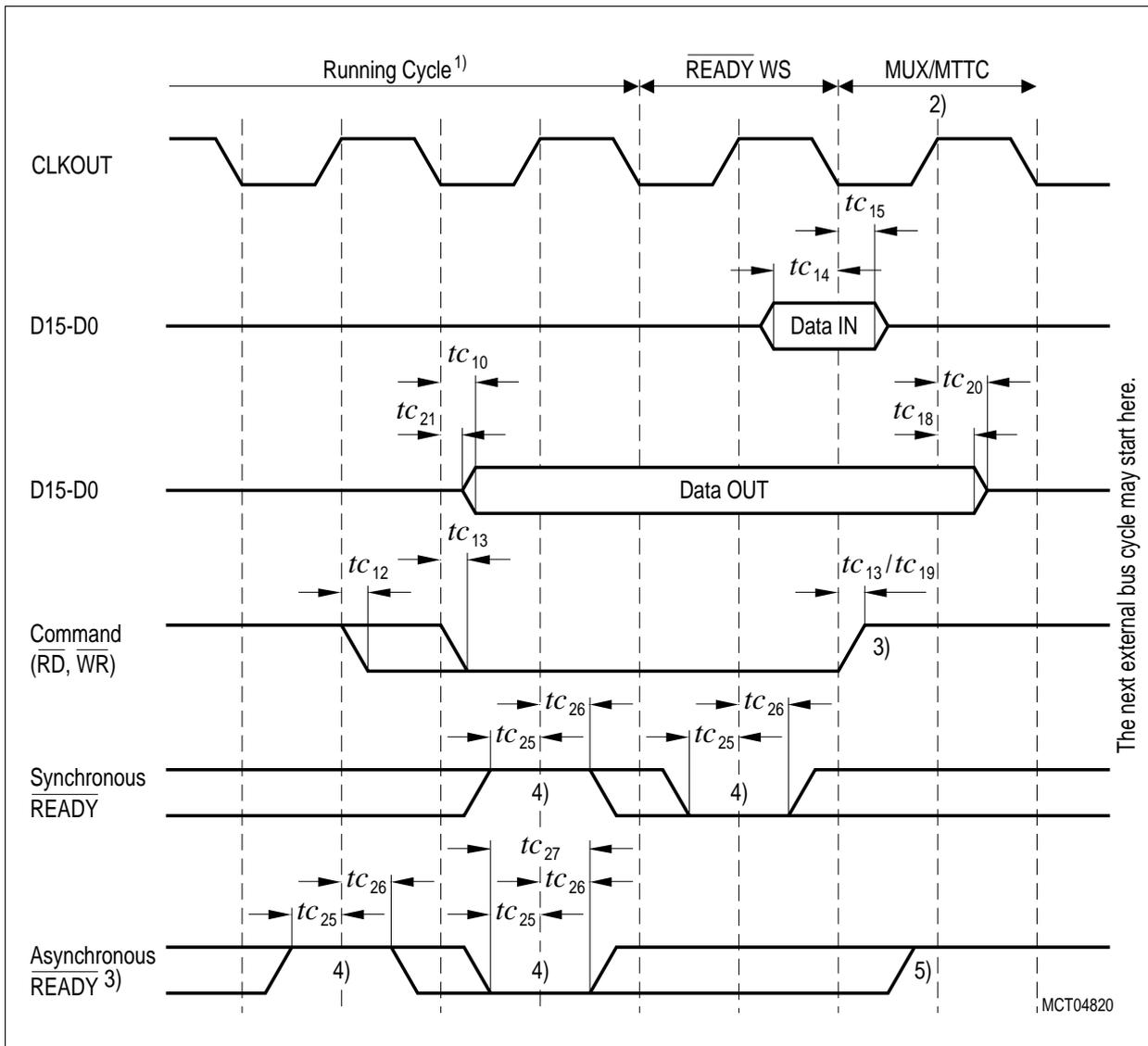
Figure 21  $\overline{\text{READY}}$  Timing
