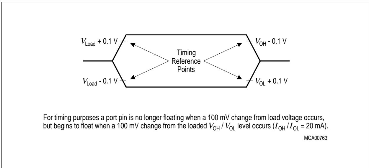
**Figure 15** Float Waveforms
