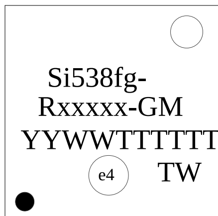
Figure 12.1. Si5381/82 Top Marking
