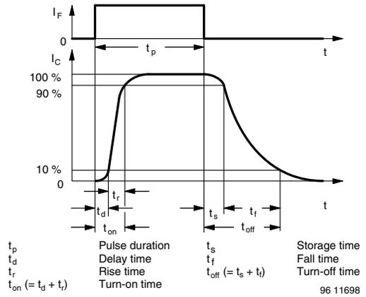
Fig. 5 - Switching Times
