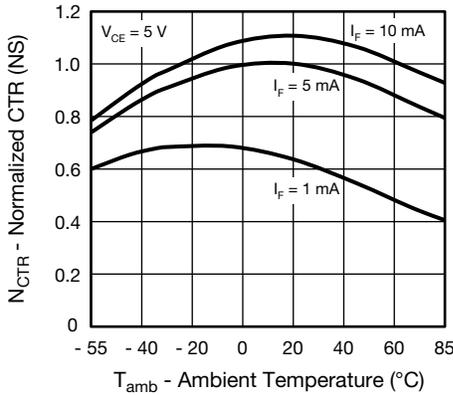
Fig. 12 - Normalized CTR (NS) vs. Ambient Temperature
