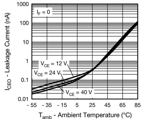
Fig. 10 - Leakage Current vs. Ambient Temperature
