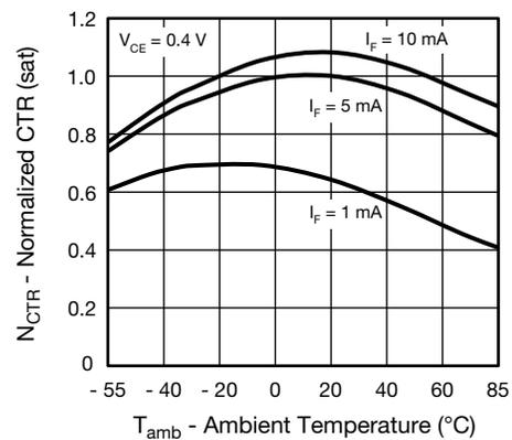
Fig. 11 - Normalized CTR (sat) vs. Ambient Temperature
