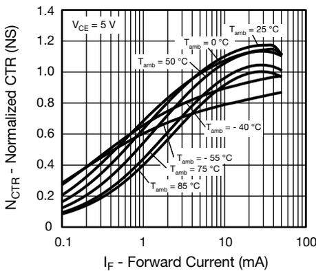
Fig. 13 - Normalized CTR (NS) vs. Forward Current
