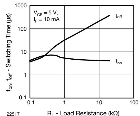
Fig. 17 - Switching Time vs. Load Resistance
