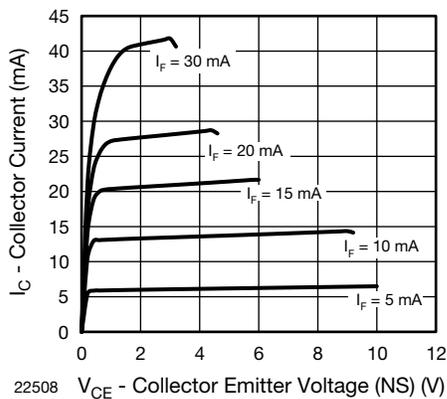
Fig. 8 - Collector Current vs. Collector Emitter Voltage (NS)
