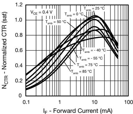
Fig. 14 - Normalized CTR (sat) vs. Forward Current
